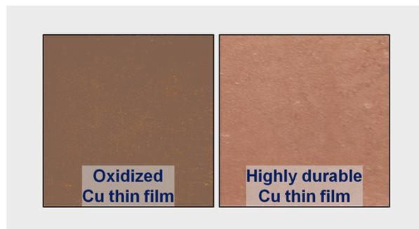
Fig. S7 The surface photo image of oxidized and highly durable Cu thin films using screen printing after 1 month at room temperature.
