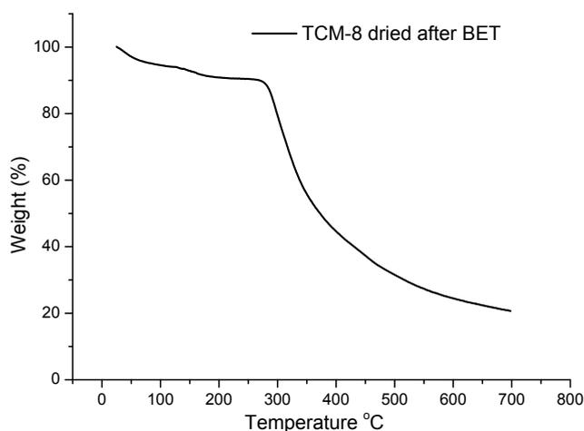
**Fig S3b:** Thermogravimetric analysis of a dried sample of **TCM-8** (used for BET analysis), heating rate 3°C/min from 25 °C to 700 °C.
