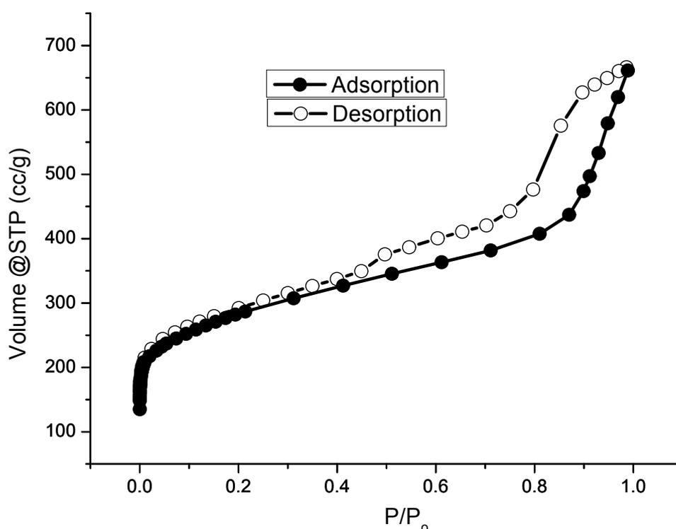
**Fig. S4:** BET analysis of **TCM-8**. Activated using CH<sub>2</sub>Cl<sub>2</sub>, dried under vacuum at 160°C.
