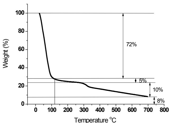
**Fig. S3a:** Thermogravimetric analysis of **TCM-8** conducted between 25 °C to 700 °C at a heating rate of 3 °C per minute.
