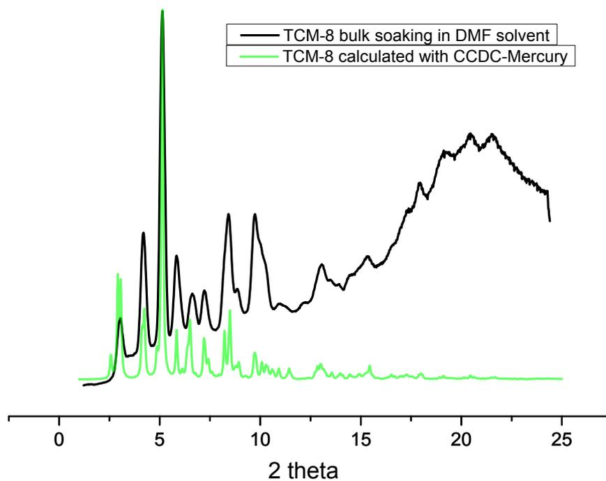
**Fig. S6a:** Powder X-ray diffraction pattern of the bulk sample of **TCM-8** (black) and its calculated pattern (green).
