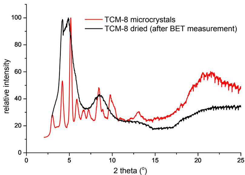
**Fig. S6b:** Powder X-ray diffraction pattern of a dried sample of **TCM-8** used for BET analysis (black line,) and a solvated microcrystalline sample of **TCM-8** (red line).
