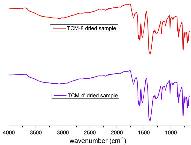
**Fig. S1:** FT-IR spectra of dried samples of **TCM-4'** and **TCM-8**.
