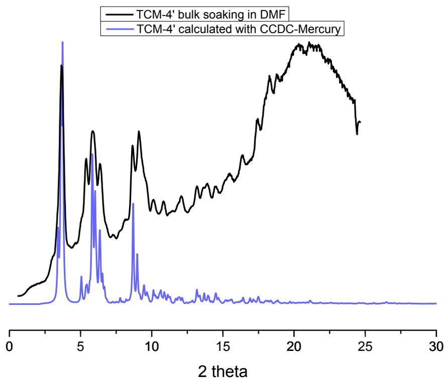
**Fig. S5:** Powder X-ray diffraction pattern of the bulk sample of **TCM-4'** (black) and its calculated pattern (blue).
