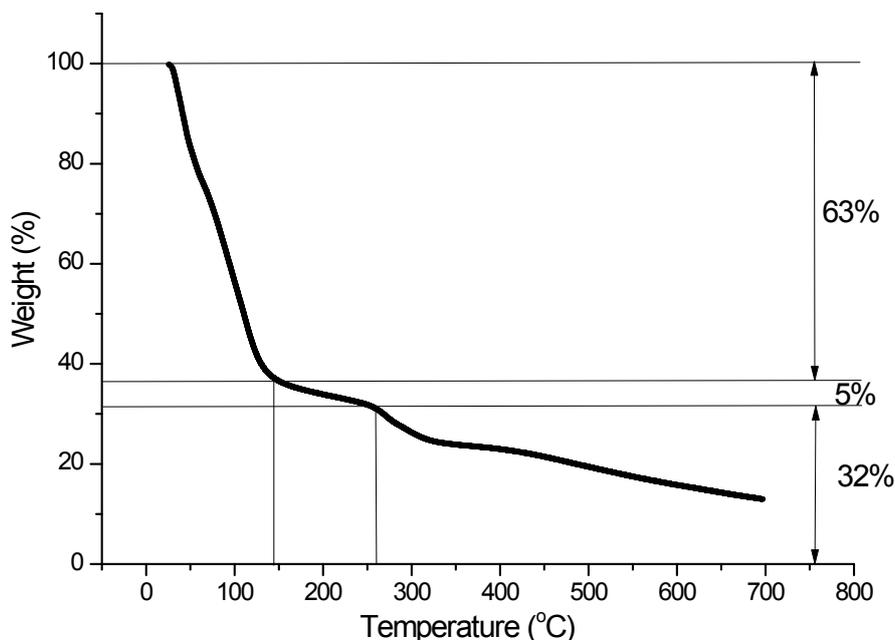
**Fig. S2:** Thermogravimetric analysis of **TCM-4'** conducted between 25°C to 700°C at a heating rate of 3°C per minute.
