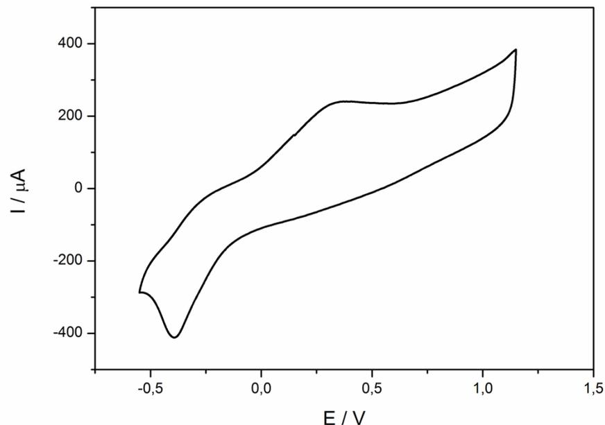
**Fig. 1.** Cyclic voltammogram at 25°C of PEDOT electrode in 0.1M  $\text{Li}(\text{CF}_3\text{SO}_2)_2\text{N}/\text{CH}_3\text{CN}$  using ITO glass, silver wire and stainless steel lattice as working, reference and counter electrodes, respectively; scan rate,  $50 \text{ mV}\cdot\text{s}^{-1}$ ; the potential (V) was referenced to the ferrocene (Fc)/ferricinium ( $\text{Fc}^+$ ) redox couple.
