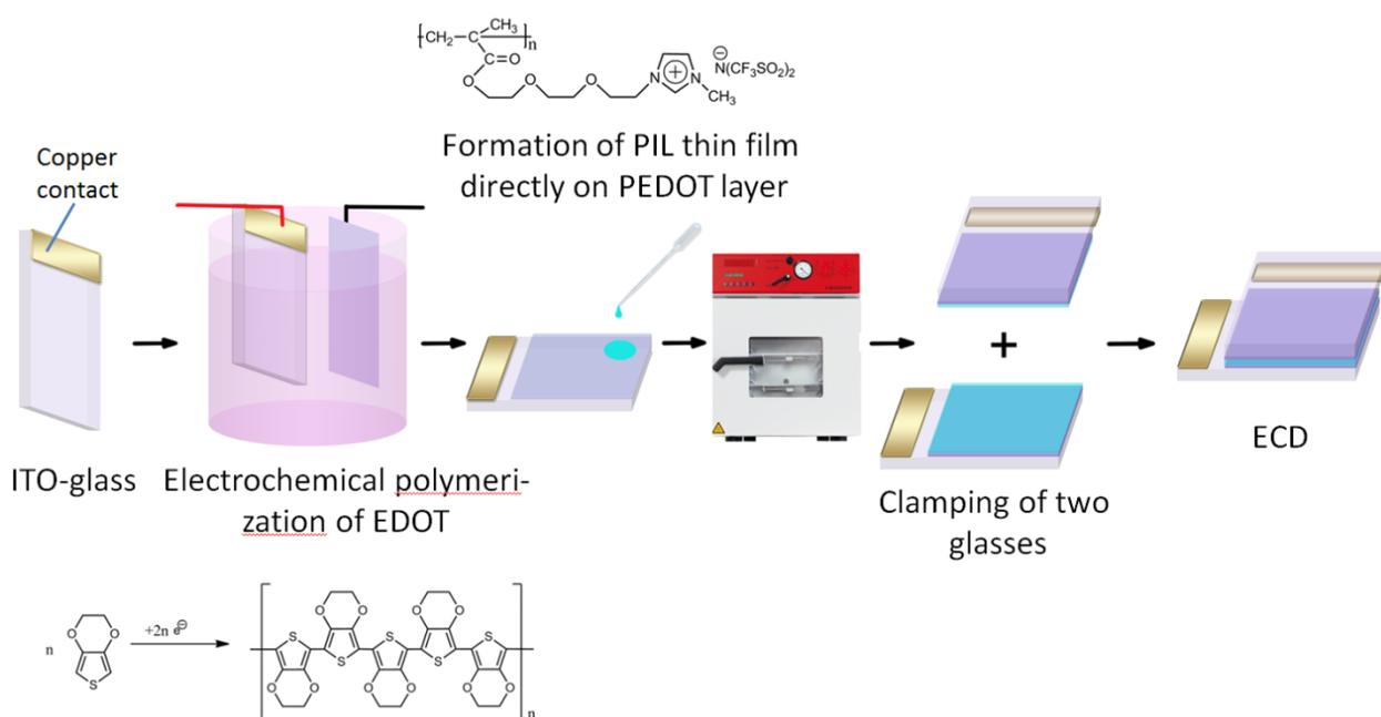
**Fig. 2.** Device assembly.
