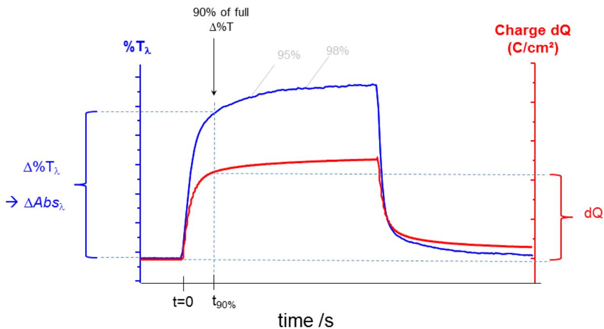
**Fig. 4.** Determination of the ECD's coloration efficiency.
