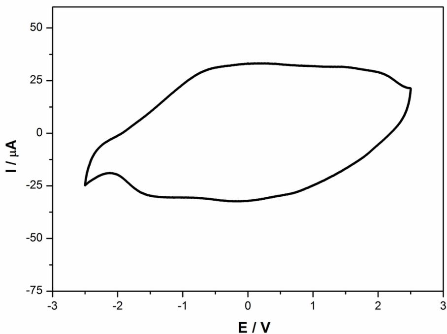
**Fig. 3.** Electrochemical characterization of symmetrical PEDOT/PIL/PEDOT electrochromic device by cyclic voltammetry at  $60 \text{ mV}\cdot\text{s}^{-1}$ .
