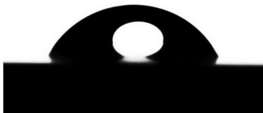
Fig. S12 Digital photograph of water droplet ( $2\ \mu\text{L}$ ) shape on untreated clean Cu surface.
