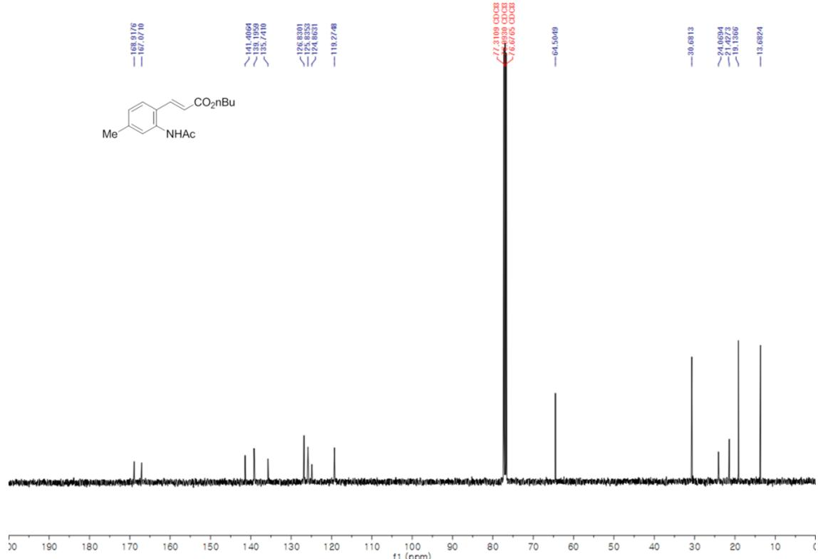
100 MHz,  $^{13}\text{C}$  NMR in  $\text{CDCl}_3$
