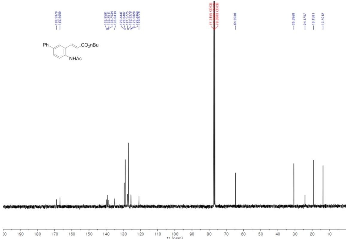
100 MHz, <sup>13</sup>C NMR in CDCl<sub>3</sub>
