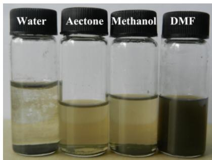
Fig. S1 Photos of the dried MoS<sub>2</sub> dispersed in solvents under sonication
