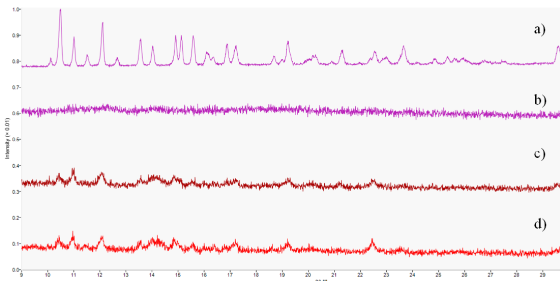
Figure S4: Comparison of the simulated (a), observed dehydrated (b), observed rehydrated after 2h (c), and observed rehydrated after 24h (d), PXRD patterns for 1 .
