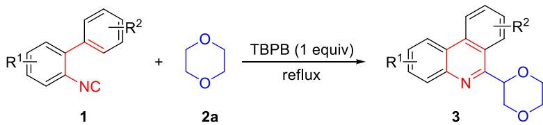
A mixture of isocyanide **1** (0.5mmol) and 1,4-dioxane (**2a**) (3 mL), TBHP (1 equiv) were added into a flask under Ar. Then the mixture was vigorously stirred under at 100 °C for 3 h (monitored by TLC). After removing the solvents in vacuo, the residue was directly purified by flash column chromatography by using ethyl acetate and petroleum ether as eluents to afford pure product **3**.
