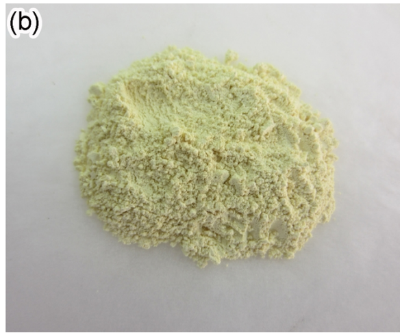
Fig. S2 (a) SEM image and (b) photograph of bulk g-C 3 N 4 powder.
