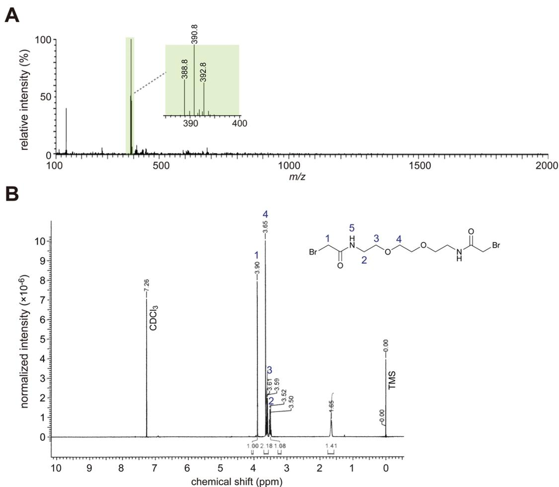
**Figure S8.** (A) MS spectrum (observed  $m/z$  values = 388.8, 390.8 and 392.8; calculated  $m/z$  values = 389.0, 341.0 and 393.0) and (B)  $^1\text{H}$  NMR spectrum of EBB.
