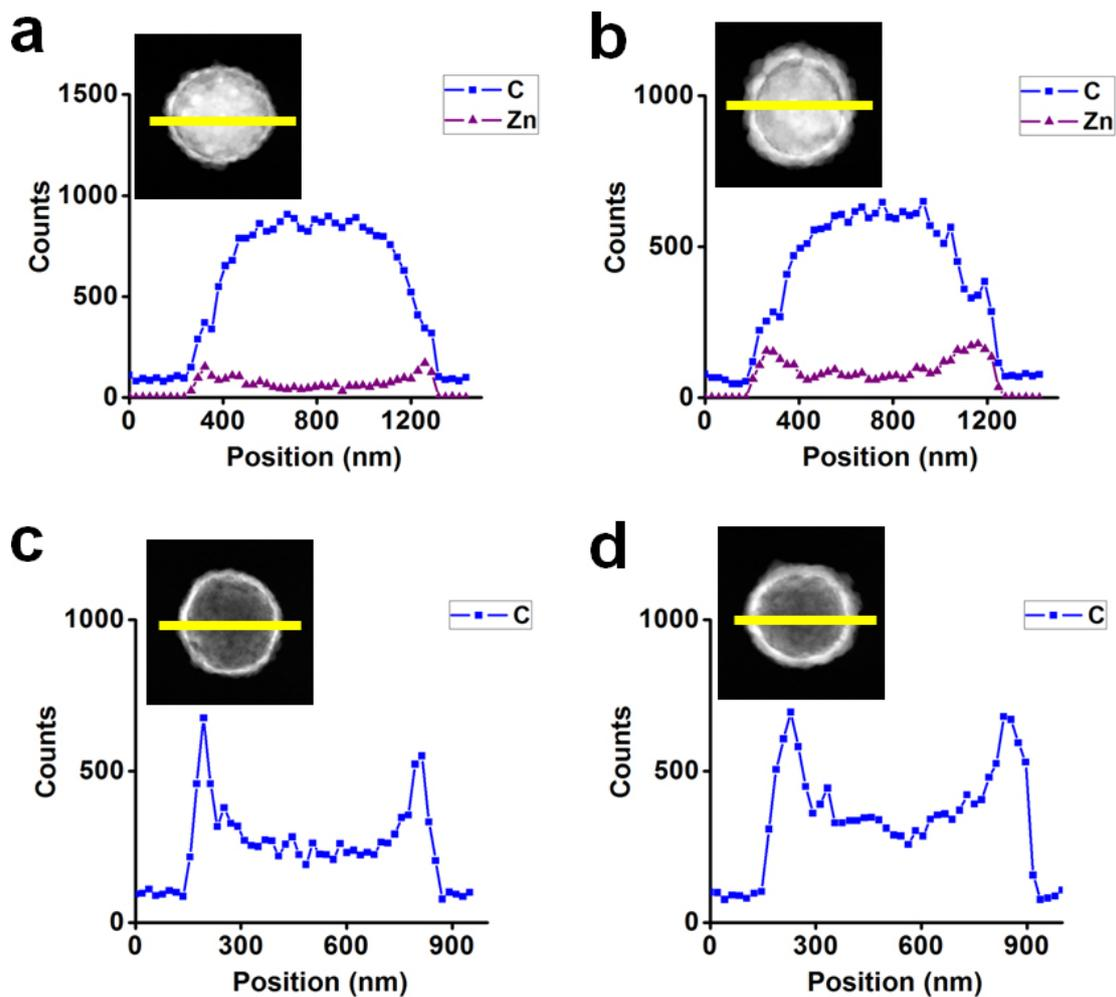
**Fig. S3** EDX spectrum profile scanning data of (a,b) polystyrene@ZIF-8 core-shell precursors, (c) **HPC-2** and (d) **HPC-3**. EDX spectrum profile scanning data were obtained by performing the scan shown in the STEM images.
