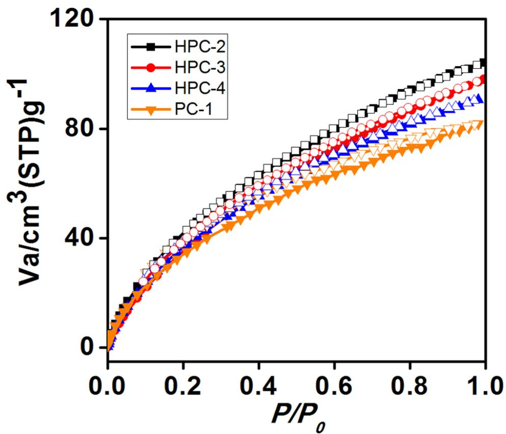
**Fig. S11** CO<sub>2</sub> sorption isotherms measured at 298 K. Solid symbols denote adsorption and open symbols denote desorption.
