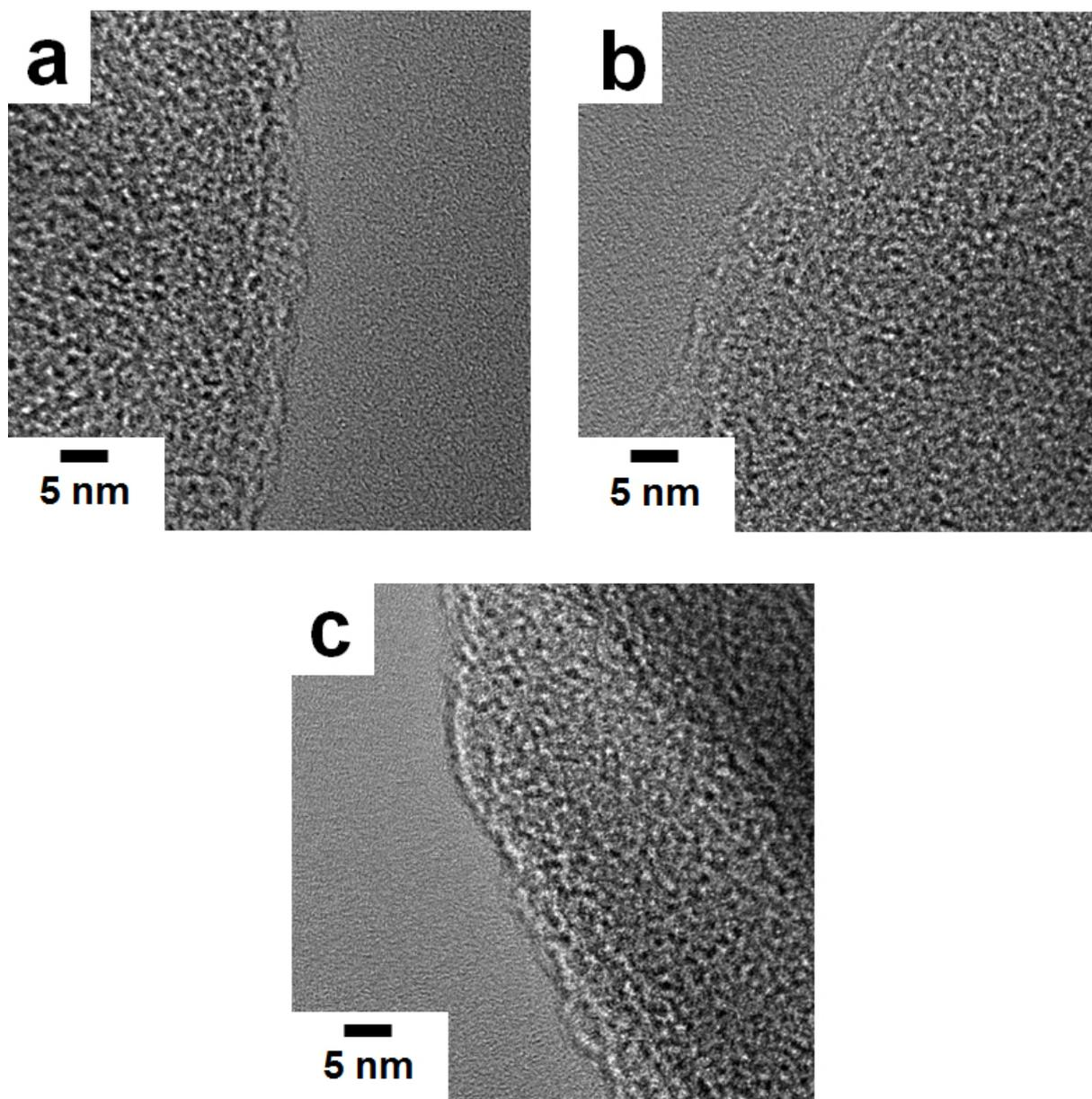
**Fig. S2** High resolution TEM (HRTEM) images of (a) **HPC-2**, (b) **HPC-3** and (c) **HPC-4**.
