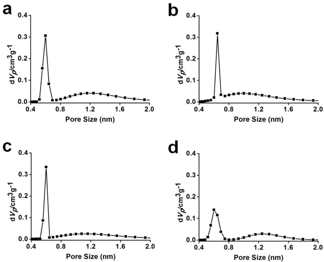
**Fig. S8** Pore size distributions of (a) **HPC-2**, (b) **HPC-3**, (c) **HPC-4** and (d) **PC-1** calculated from the NLDFT (non local density function theory) method.
