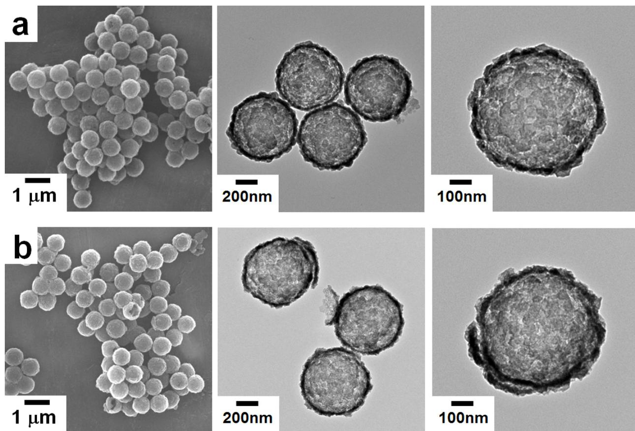
**Fig. S9** SEM and TEM images of hollow porous carbons obtained a pyrolysis at (a) 800 °C and (b) 900 °C.
