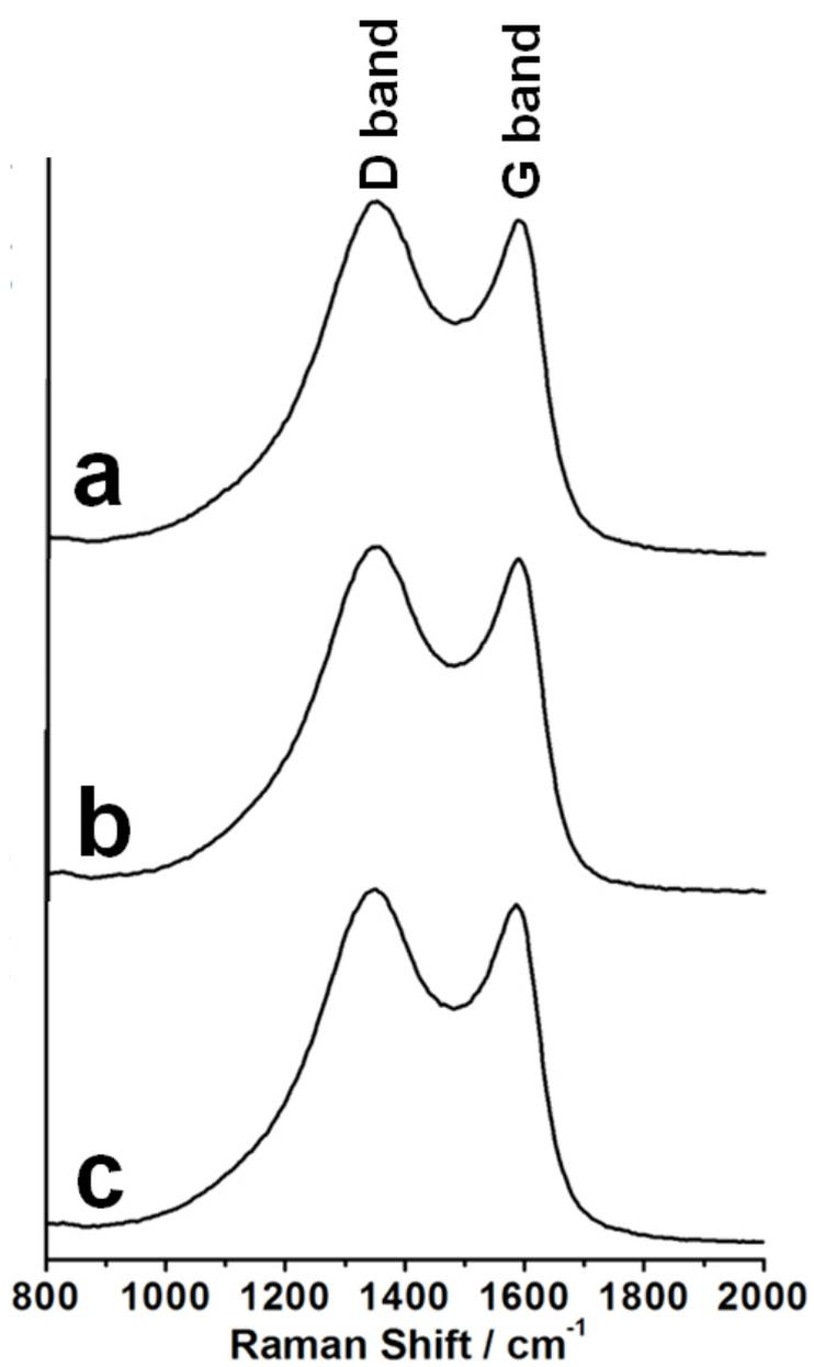
**Fig. S6** Raman spectra of (a) HPC-2, (b) HPC-3 and (c) HPC-4.
