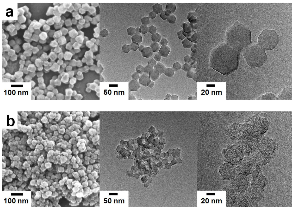
**Fig. S7** SEM and TEM images of (a) nano-sized ZIF-8 particles and (b) **PC-1** obtained from the pyrolysis of nano-sized ZIF-8 particles.
