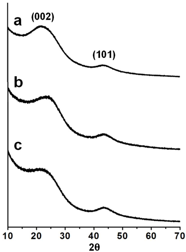
**Fig. S5** PXRD patterns of (a) HPC-2, (b) HPC-3 and (c) HPC-4.
