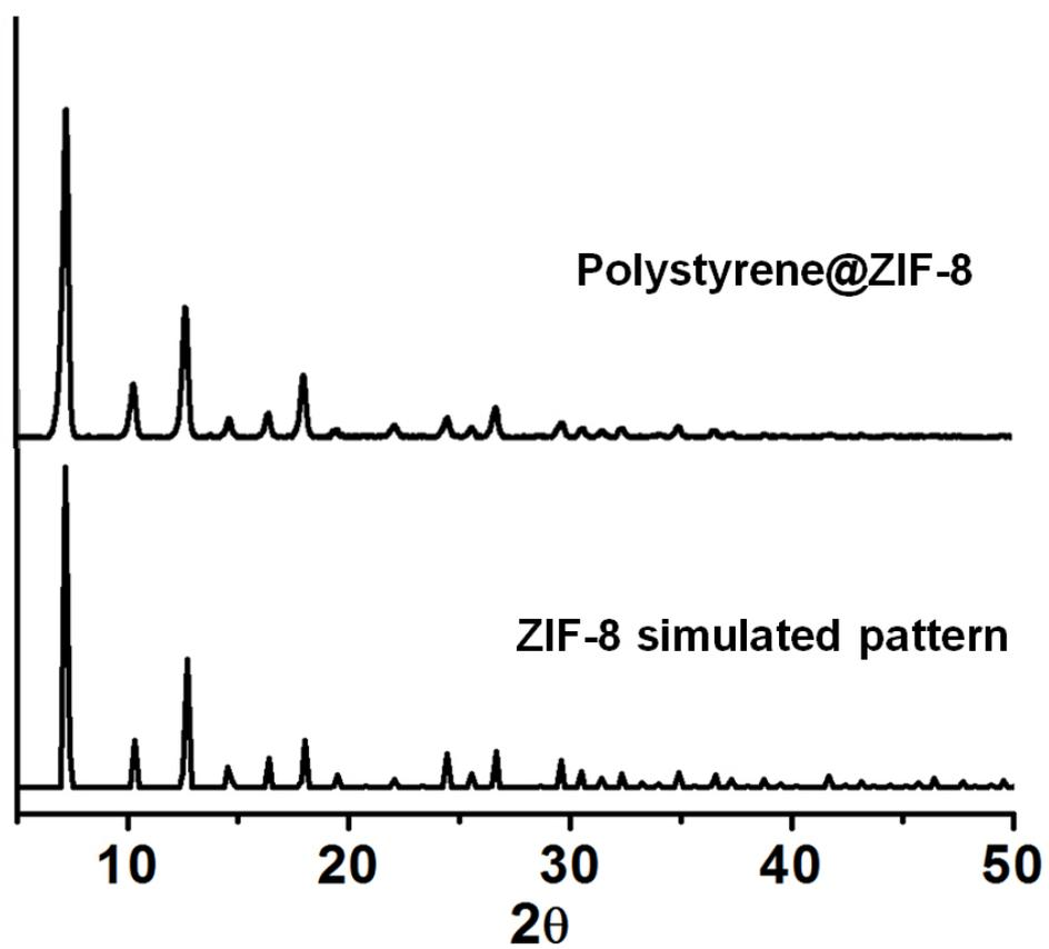
**Fig. S4** PXRD patterns of polystyrene@ZIF-8 core-shell microspheres (up) and the simulated pattern of ZIF-8 (down).
