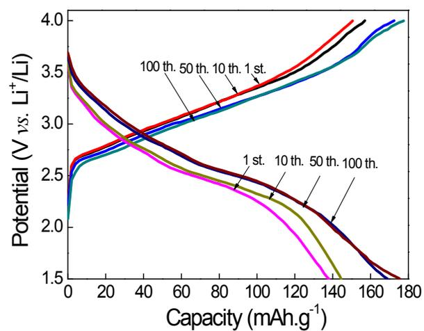
Figure S9 The corresponding charge/discharge profile of “nanocross” cycled at 3.05 A.g<sup>-1</sup>.
