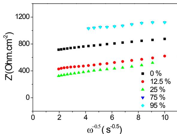
Figure S8 Comparison of  $Z'-\omega^{-0.5}$  plot of hierarchical VOx with different water content.
