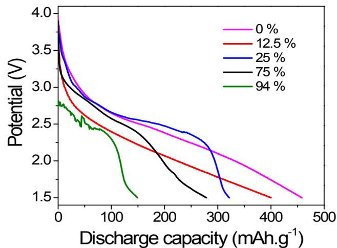
Figure S5 Corresponding discharge profiles of the initial cycle of  $\text{VO}_x$  hierarchical structures.
