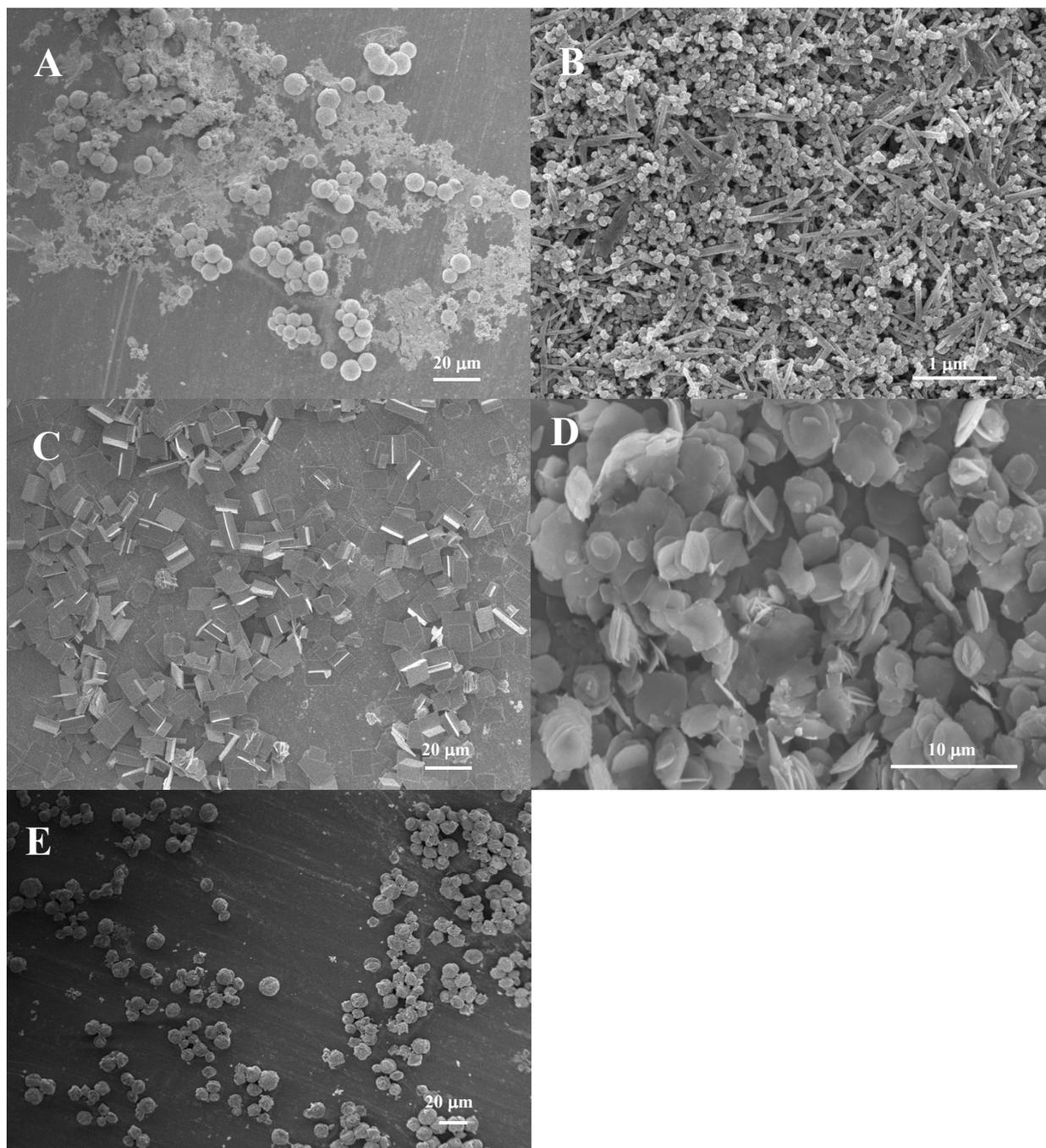
Figure S1 Low magnification SEM images of hierarchical VO<sub>x</sub> with (A) 0%, (B) 12.5 %, (C) 25 %, (D) 75 % and (E) 95 % water content.
