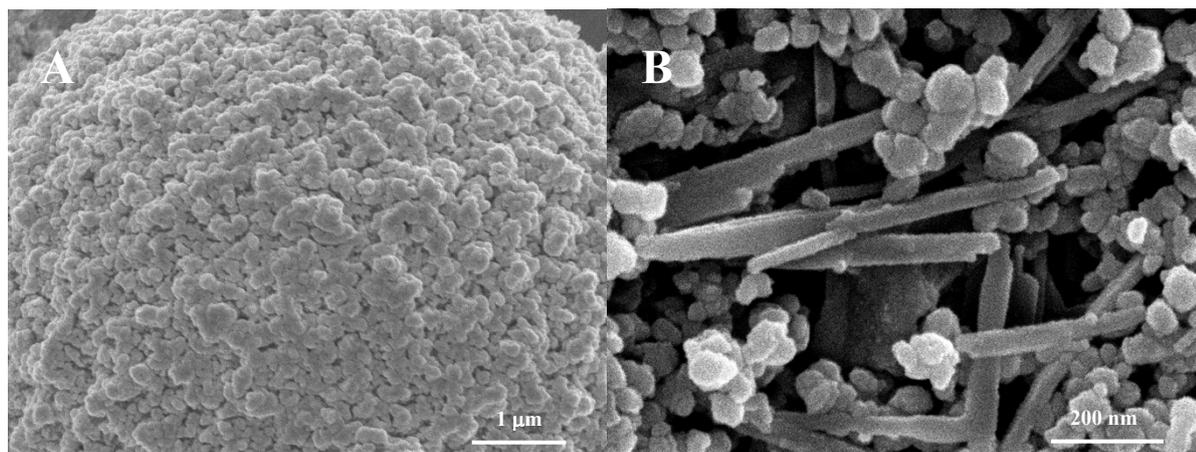
Figure S2 High magnification SEM images of hierarchical VO<sub>x</sub> with (A) 0% and (B) 12.5 % water content.
