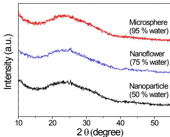
Figure S4 Crystallinity characterization of  $\text{VO}_x$  hierarchical structure with 50 %, 75 % and 95% water content.
