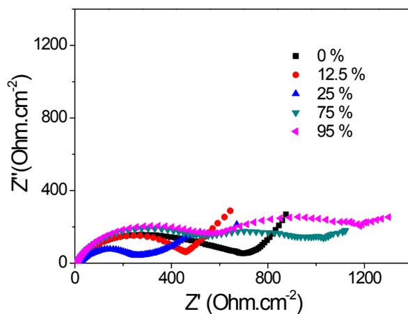
Figure S7 EIS tests of hierarchical VO<sub>x</sub> with different water content after 100 cycles at 0.05 A.g<sup>-1</sup>.
