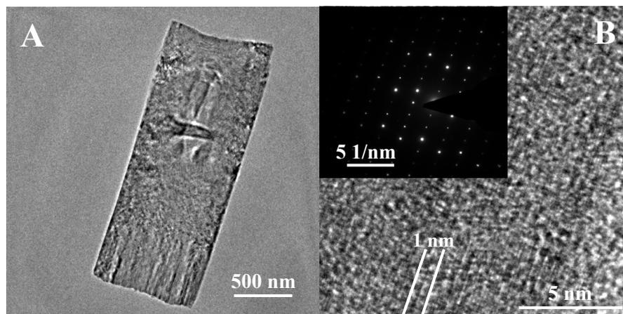
Figure S3 TEM images of V<sub>4</sub>O<sub>7</sub> “nanocross” with (A) low resolution TEM image; (B) high resolution TEM image and SAED pattern inset.
