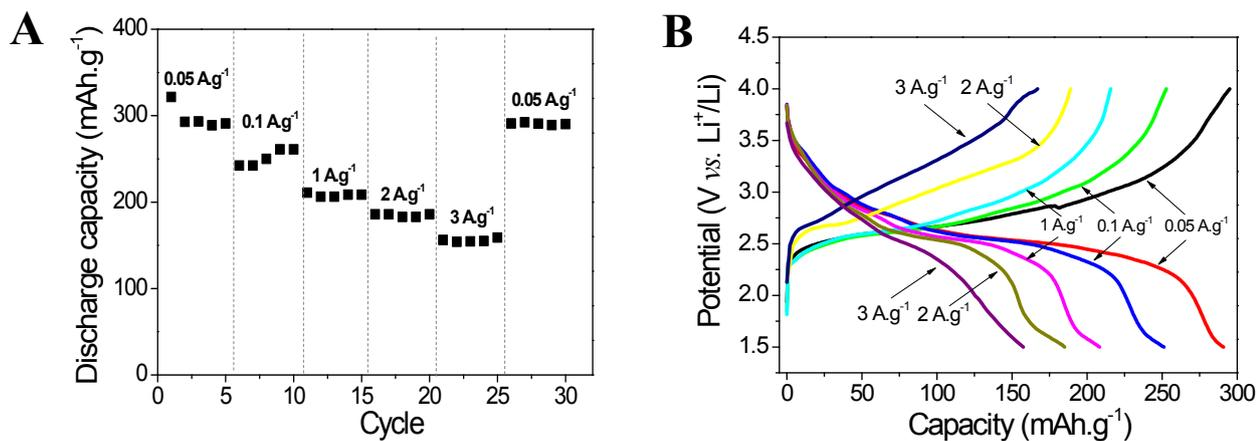
Figure S6 Rate performance of “nanocross” V<sub>4</sub>O<sub>7</sub> with (A) different current density and (B) corresponding charge/discharge profile.
