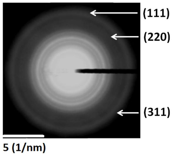
**Fig. S1** SAED pattern of Mn<sup>2+</sup>-doped ZnS QDs with the Miller indexes indicated.
