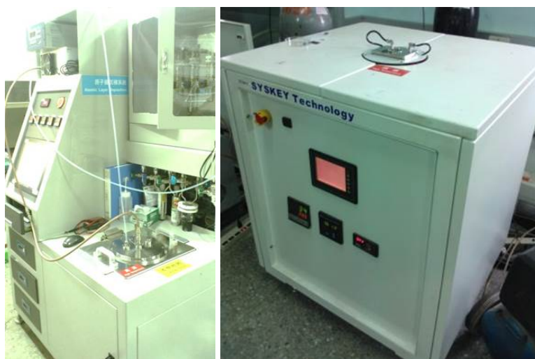
Fig. 1 Photographs of the home-made ALD systems.
