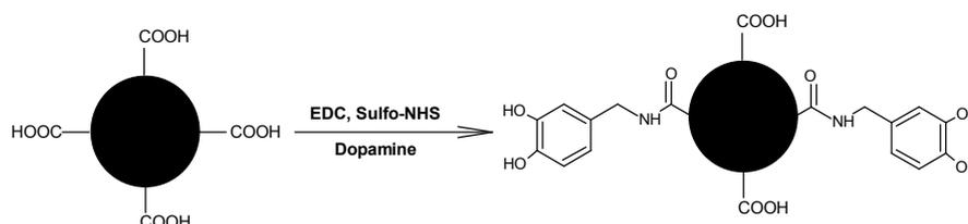
**Scheme S1** Representation for partial derivatisation of carboxyl coated CNPs with dopamine.
