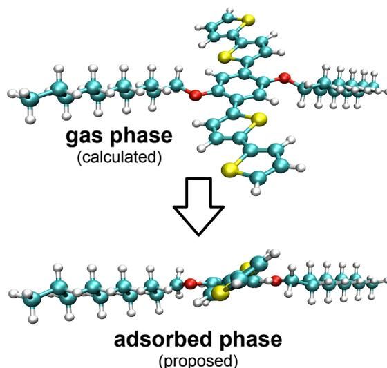
Figure S3: Optimized geometry for gas phase DTB10B molecule obtained at DFT/B3LYP/6-31G level, and the subsequent planarization upon its adsorption on the Si(111)-B surface. The geometry of the adsorbed phase was not optimized but was adjusted during STM simulations to reproduce the main experimental STM features.
