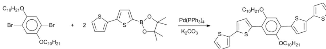
Figure S1: Synthesis of 1,4-bis(2',2''-dithienyl)-2,5-bis(decyloxy)benzene, DTB10B
