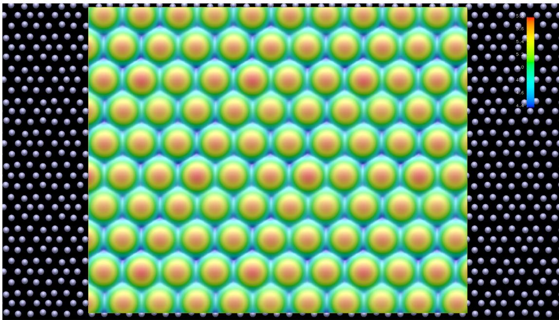
Figure S4: Calculated topographic STM image for the Si(111)-B surface containing 5733 atoms, dimension of the Si(111)-B model =  $13.8 \text{ nm} \times 13.6 \text{ nm} \times 0.5 \text{ nm}$ . STM simulations conditions: EHT Hamiltonian, Tersoff-Hamann method,  $I = 0.1 \text{ nA}$ ,  $V = 2 \text{ V}$ , scanned zone =  $(6.7 \times 11.5) \text{ nm}^2$ , resolution =  $0.01 \text{ nm}$ .
