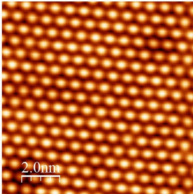
Figure S2: STM image of a clean Si(111)-B surface. Measurement conditions:  $I=0.2$  nA,  $V = 2.6$  V,  $10$  nm  $\times$   $10$  nm
