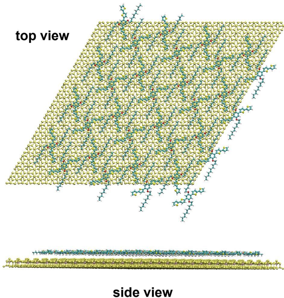
Figure S5: Molecular model used for the STM simulations of the DTB10B/Si(111)-B system. Although this supercell contains 6592 atoms, no periodic boundary conditions were applied in the STM simulation; every single atoms can be manually displaced or its chemical nature changed, while a new STM image can be subsequently evaluated.
