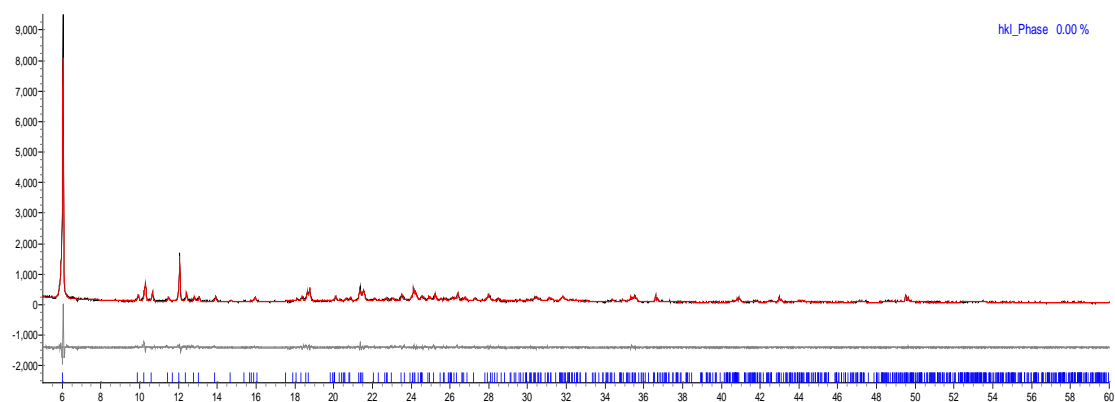
Figure S6. PXRD pattern of 2 refined by TOPAS software. R_{wp} = 11.89\% . Cell parameters: P-1 , a = 9.168 \text{ \AA} , b = 9.244 \text{ \AA} , c = 15.159 \text{ \AA} , \alpha = 87.928^\circ , \beta = 76.523^\circ , \gamma = 75.696^\circ , V = 1210.3 \text{ \AA}^3 .
