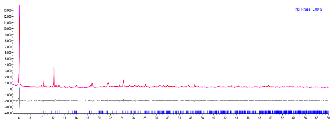
Figure S5. PXRD pattern of 1 refined by TOPAS software. R_{wp} = 8.76\% . Cell parameters: P-1 , a = 9.159 \text{ \AA} , b = 9.247 \text{ \AA} , c = 15.160 \text{ \AA} , \alpha = 87.934^\circ , \beta = 76.555^\circ , \gamma = 75.622^\circ , V = 1209.4 \text{ \AA}^3
