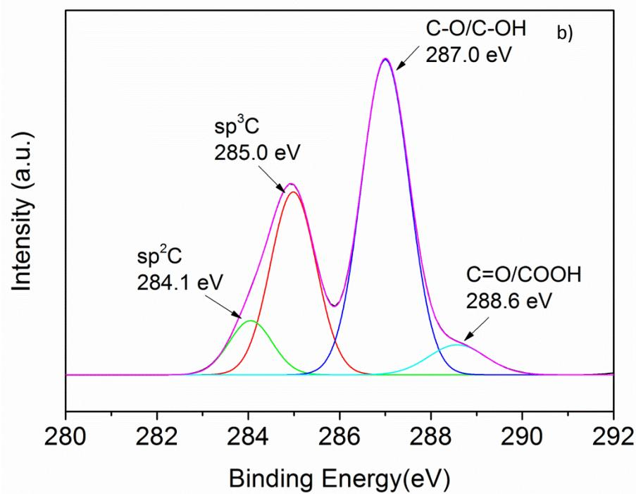
**Fig. S3** Curve-fitting of C1s XPS spectra of a) 3DGO and b) 2DGO
