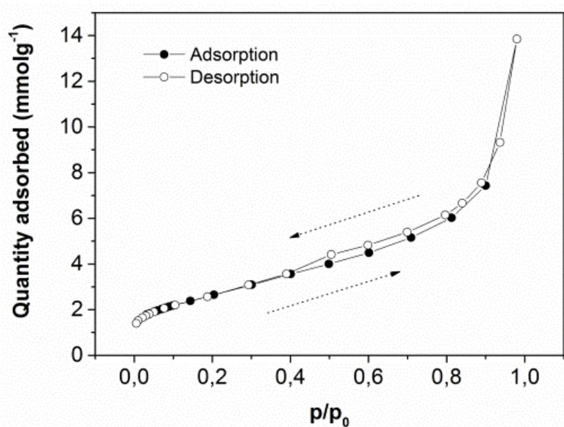
Fig. S1 Nitrogen adsorption-desorption isotherm of 3DGO.
