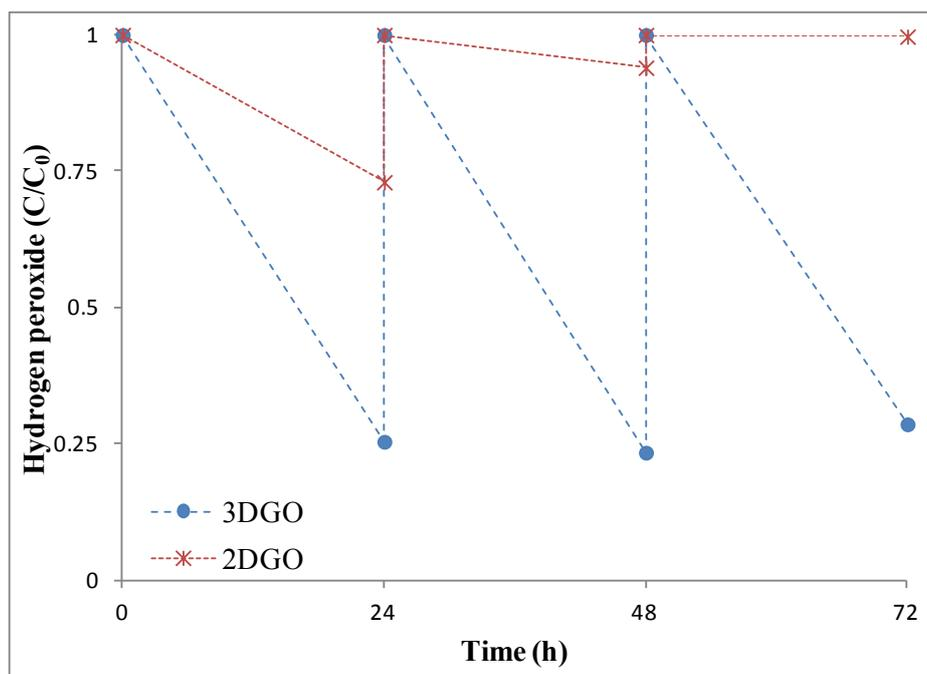
**Fig. S4** Determination of hydrogen peroxide amounts during the catalytic reactions, both for 2D and 3DGO. For the determination of  $H_2O_2$ , aliquots of each reaction were dissolved in dilute sulphuric acid cooled with ice and  $H_2O_2$  was titrated against 0.1 N ceric sulfate solution, using ferroin as indicator [1].
