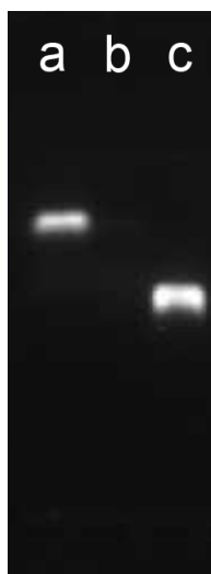
Fig. S5 PAGE analysis of 1.0 \mu\text{M} probe (lane a), 1.0 \mu\text{M} probe treated with 75 \mu\text{g mL}^{-1} GO for 2 min (lane b) and 1.0 \mu\text{M} probe firstly hybridized with 1.0 \mu\text{M} target at 37 ^{\circ}\text{C} for 10 min and subsequently treated with 75 \mu\text{g mL}^{-1} GO for 2 min (lane c).
