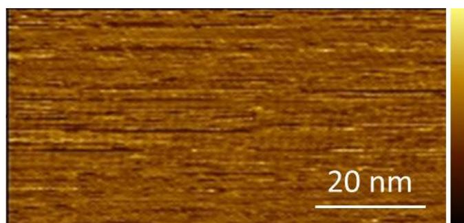
Fig. S4 Typical STM image of benzenethiol-modified Au(111) taken by the AgNW-tip. The colour bar: 0 – 4 nm (constant current mode at 1 nA and 0.1 V).
