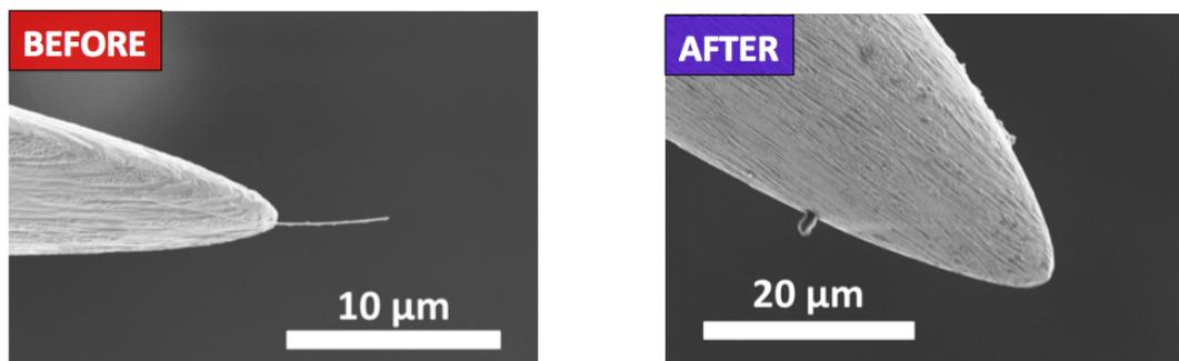
Fig. S2 SEM images of the AgNW-tip, that is attached with only single NW, before (left) and after (right) STM scanning.
