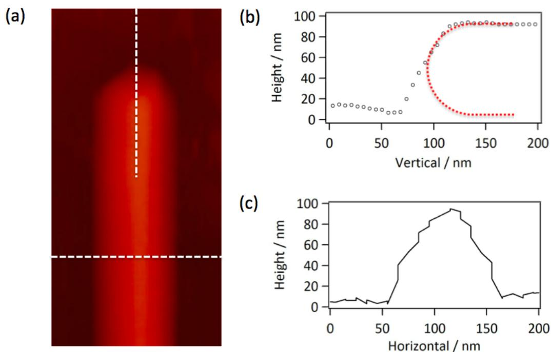
Fig. S3 (a) Typical STM topographic image of the AgNWs used in this study; (b) line profile at the end of the NW along the vertical white dashed line in (a); (c) Line cross section of the NW along the horizontal white dashed line in (a).
