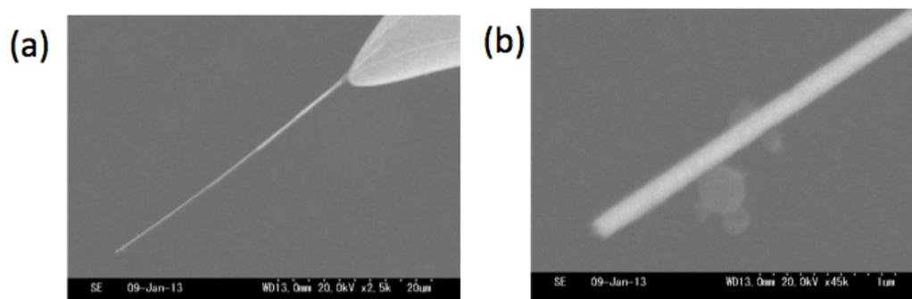
Fig. S1 SEM images of the AgNW-tip shown in Fig. 1 after STM scanning
