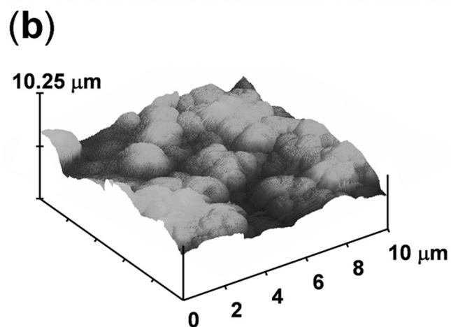
**Supporting Figure 2.** Surface topography of the *f*-DOPA-coated gold substrate: (a) FE-SEM and (b) AFM micrographs.
