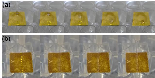
**Supporting Figure 3.** Photographs for the manipulation of water droplets and flow on the slightly tilted *f*-DOPA-coated gold substrate: (a) the capture of a sliding water droplet at the relatively hydrophilic area (dotted square) and (b) the control of water flow. The dotted line is the relatively hydrophilic area surrounded by superhydrophobic areas.
