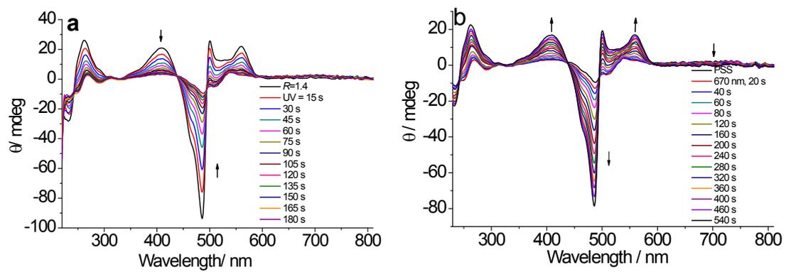
**Fig. S20** CD spectral change of **1**/AT10 in binding mode I ( $C_1 = 1.4 \times 10^{-5}$  M,  $R = 1.4$ ) with successive irradiation of (a) UV and (b) 670 nm light at room temperature.
