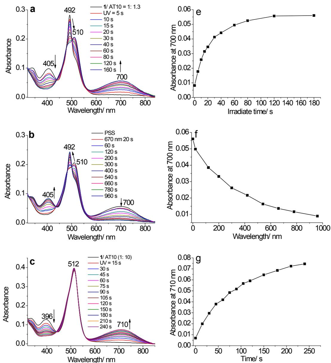
**Fig. S16** The absorption spectral change of **1** ( $5.0 \times 10^{-6}$  M) in the presence of DNA with a molar ratio of  $R = 1.3$  with alternate irradiation of (a) UV and (b) visible light; and a molar ratio of  $R = 10.0$  with irradiation of (c) UV light; the related absorbance change at 700 nm (710 nm for (g)) vs irradiation time for (a), (b) and (c) are shown in (e), (f) and (g), respectively.
