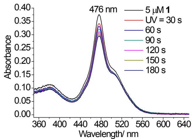
**Fig. S5** The absorption spectra of **1** ( $5.0 \times 10^{-6}$  M) in water with irradiation of UV light.
