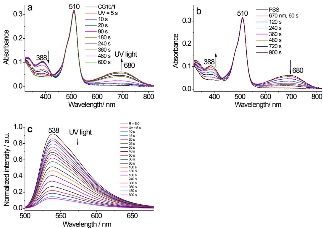
**Fig. S18** The absorption change of CG10/1 ( $R = 3.0$ ) with (a) UV light irradiation and (b) the PSS state with 670 nm light irradiation. (c) The fluorescence change of  $R = 6.0$  with UV light irradiation.  $\lambda_{ex} = 480$  nm,  $\lambda_{em} = 540$  nm.
