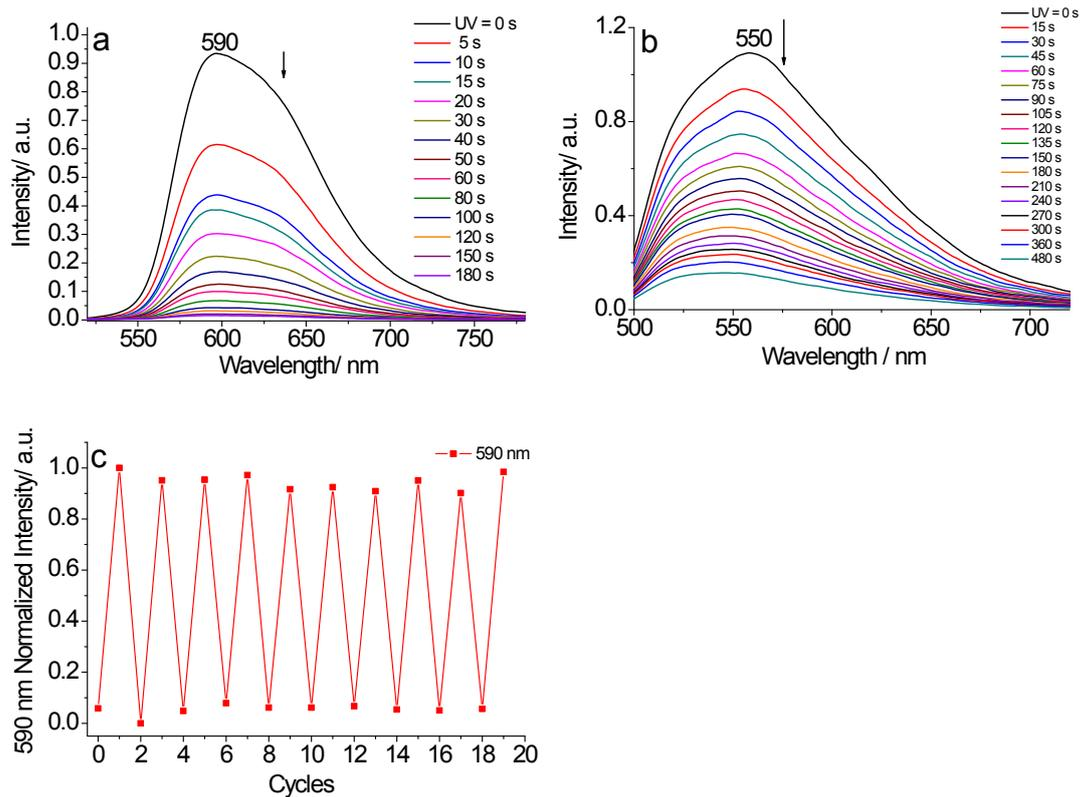
**Fig. S17** The emission spectral change of AT10/1 ( $C_1 = 5.0 \times 10^{-6}$  M) with (a)  $R = 1.3$  and (b) 10.0 with UV light irradiation. (c) The change of emission intensity at 590 nm at intervals of UV and 670 nm light irradiation under the condition of  $R = 1.3$ .
