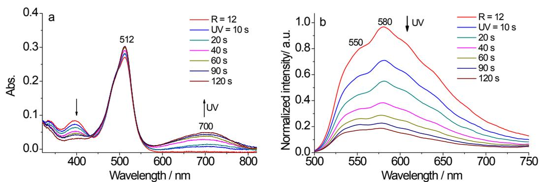
**Fig. S19** The absorption and emission ( $\lambda_{ex} = 480$  nm) change of CtDNA/1 ( $R = 12$ ) with UV irradiation.
