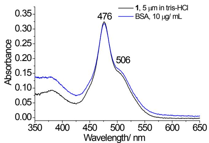
**Fig. S15** The absorption spectra of **1** ( $5.0 \times 10^{-6}$  M) in water in the presence of 10  $\mu\text{g/mL}$  BSA (Bovine serum albumin) with irradiation of UV light.
