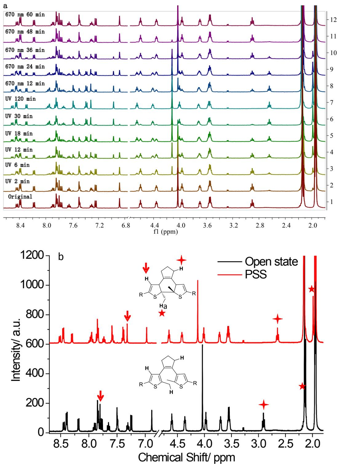
**Fig. S4**  $^1\text{H}$  NMR spectra of **1** (a) alternately irradiated with UV and 670 nm laser light for different period of time in acetonitrile- $d_3$  solution ( $1.2 \times 10^{-3}$  M) and (b) the open and PSS state of **1** in acetonitrile- $d_3$  at room temperature.
