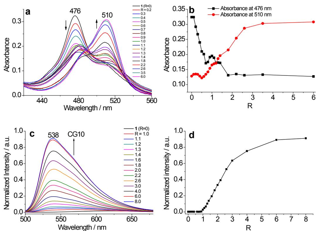
**Fig. S11** (a) The absorption spectra of CG10/1 ( $5.0 \times 10^{-6}$  M in aqueous buffer solution, pH = 7.2) with increasing concentration of CG10 ( $R = 0 - 6.0$ ) and (b) the absorbance change at 476 and 510 nm with different  $R$  value. (c) The fluorescent spectra of 1 ( $5.0 \times 10^{-6}$  M) with increasing concentration of CG10 ( $R = 0-8.0$ ) and (d) the change of fluorescent intensity at the wavelength of 538 nm with different  $R$  value.
