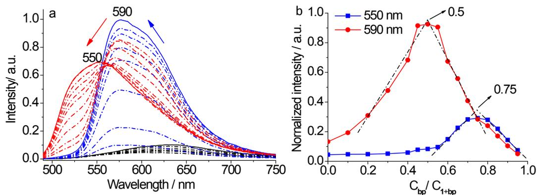
**Fig. S10** (a) The emission spectral change of AT10/1 with increasing concentration of AT10 ( $R = 0-10$ ) (solid black line: sole 1, solid blue line: binding I ( $R=1.6$ ), solid red line: bonding II ( $R = 10$ )); (b) the Job's plot of AT10/1 by fluorescent intensity change at 590 (red) and 550 (blue) nm, the black dot dash line is the linear fitting of the curve.
