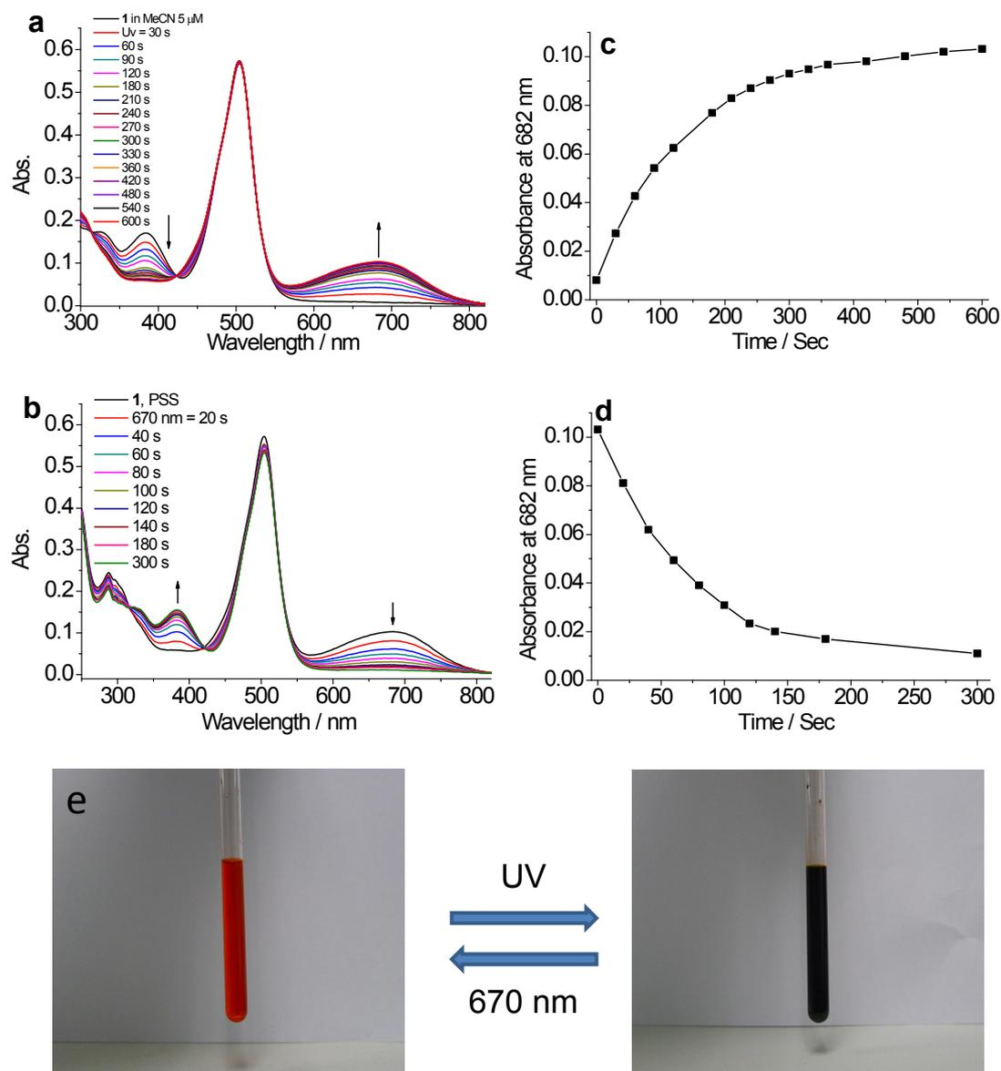
**Fig. S3** The absorption spectral change of **1** ( $5.0 \times 10^{-6} \text{ M}$  in acetonitrile) with alternate (a) UV and (b) 670 nm light irradiation; the absorption change at 670 nm with the irradiation time of UV (c) and 670 nm (d) light, 1 cm cell, at room temperature; (e) images of the open and closed form of **1** in acetonitrile- $\text{d}_3$  solution ( $1.2 \times 10^{-3} \text{ M}$ ) before and after UV light irradiation.
