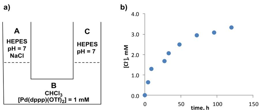
**Figure S12.** a) Schematic representation of the U-tube transport experiment. A chloroform phase (B) containing **1** (1 mM) separates two water phases. The source water phase (A) is buffered with HEPES at pH = 7 and contains NaCl 100 mM. The receiving water phase (C) contains only HEPES at pH 7. b) Variation of the chloride concentration in the receiving phase with time.
