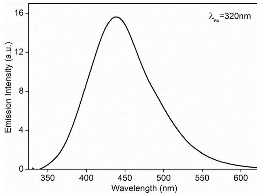
**Figure S7:** Emission spectra of MOF (**1'**) dispersed in water upon excitation at 320 nm.
