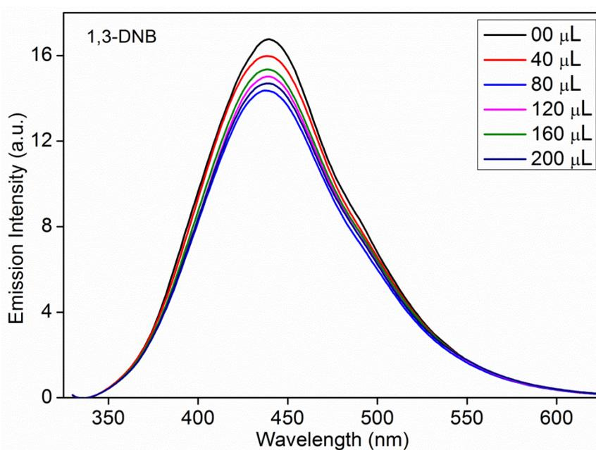
**Figure S12:** Emission spectra of MOF (**1'**) dispersed in water upon incremental addition of 1,3-DNB solution (1mM) in water.
