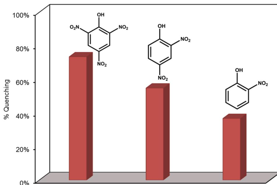
**Figure S21:** Comparison of percentage fluorescence quenching obtained upon addition of NP, 2,4-DNP, TNP to **1'** dispersed in water.
