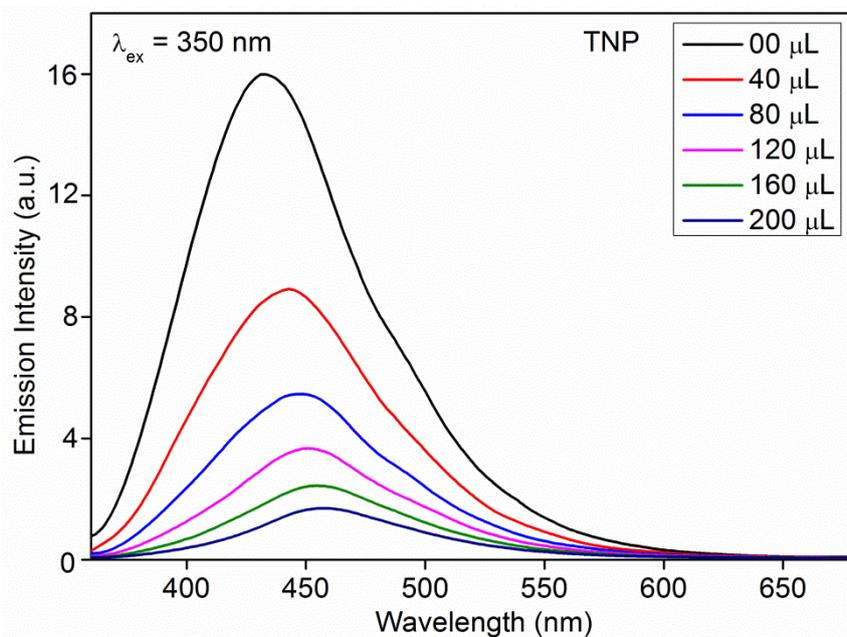
**Figure S24:** Change in the fluorescence intensity of **1'** in water upon incremental addition of aqueous TNP solution 1 mM. ( $\lambda_{ex} = 350$ ,  $[1'] = 0.5 \text{ mg/mL}$ ).
