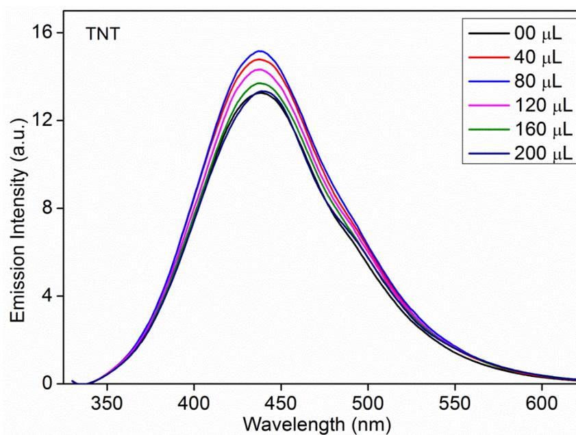
**Figure S8:** Emission spectra of MOF (**1'**) dispersed in water upon incremental addition of TNT solution (1mM) in water.
