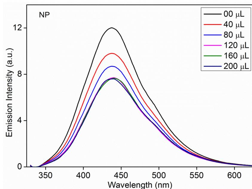
**Figure S20:** Emission spectra of MOF (1') dispersed in water upon incremental addition of NP solution (1mM) in water.
