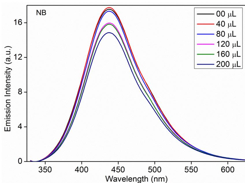
**Figure S13:** Emission spectra of MOF (**1'**) dispersed in water upon incremental addition of NB solution (1mM) in water.
