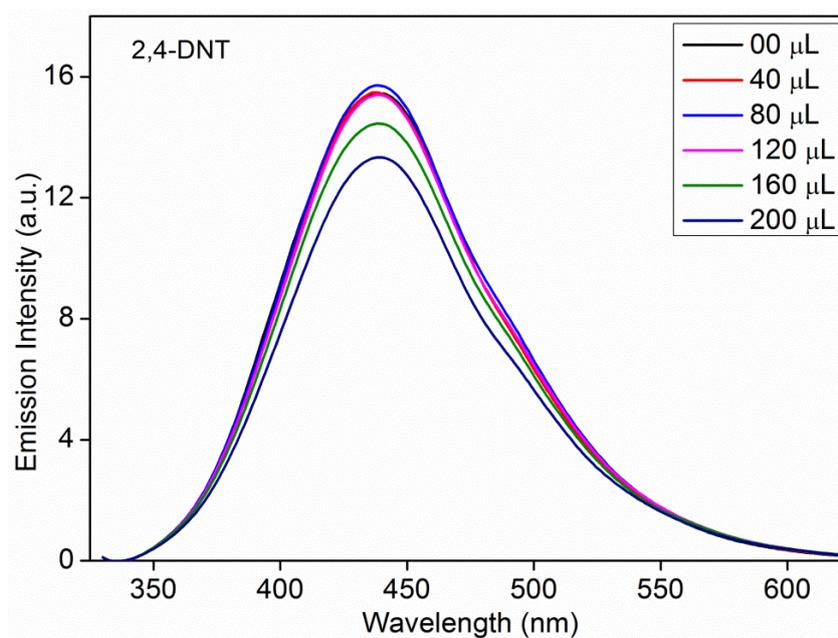
**Figure S10:** Emission spectra of MOF (**1'**) dispersed in water upon incremental addition of 2,4-DNT solution (1mM) in water.
