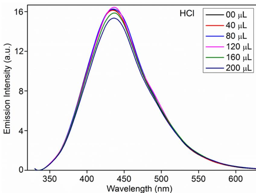
**Figure S16:** Emission spectra of MOF (**1'**) dispersed in water upon incremental addition of HCl solution (1mM) in water.
