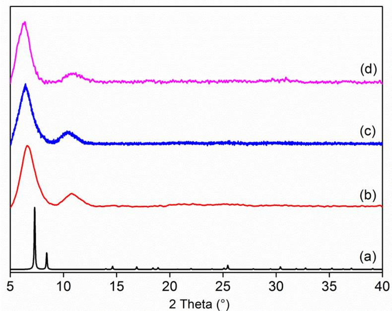
**Figure S5:** Powder X-ray diffraction patterns (PXRD) of (a) Simulated; (b) Assynthesized compound; (c) MeOH exchange MOF; (d) Desolvated MOF (1').
