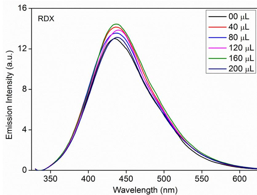
**Figure S9:** Emission spectra of MOF (**1'**) dispersed in water upon incremental addition of RDX solution (1mM) in water.
