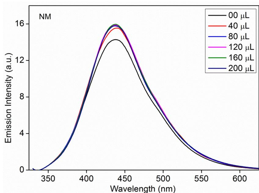
**Figure S15:** Emission spectra of MOF (**1'**) dispersed in water upon incremental addition of NM solution (1mM) in water.
