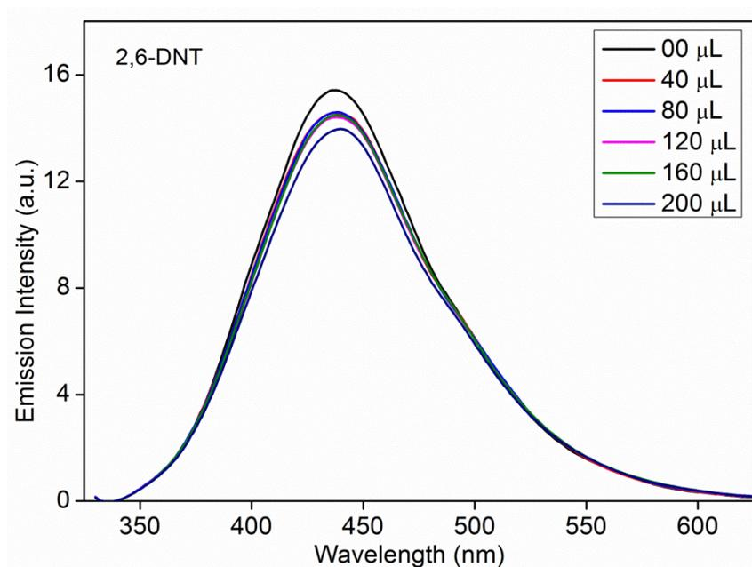
**Figure S11:** Emission spectra of MOF (**1'**) dispersed in water upon incremental addition of 2,6-DNT solution (1mM) in water.
