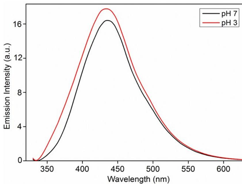
**Figure S17:** Effect of pH on fluorescence intensity of MOF (**1'**) dispersed in water.
