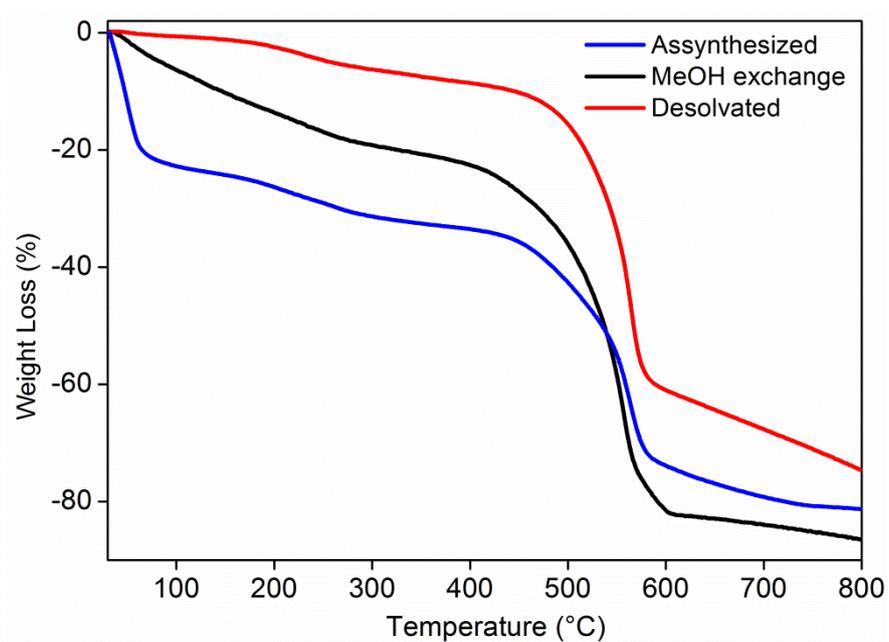
**Figure S6:** Thermo gravimetric analysis of MOF.
