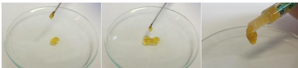
Figure 2 Behavior of the viscosity of hydrogel 5 upon mechanical stress.
