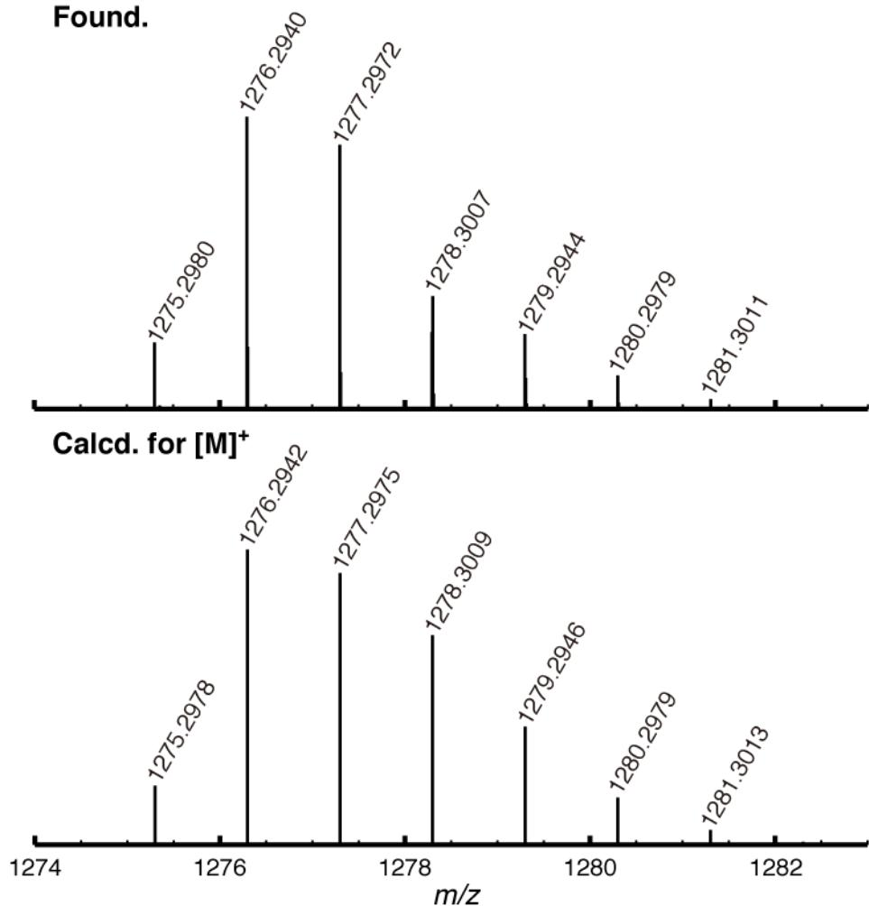
**Figure S1.** Observed high-resolution mass spectrum (top) of **1S** and the theoretical isotropic distribution pattern for  $C_{84}H_{42}BClN_6O_6$  ( $[M]^+$ ) (bottom).
