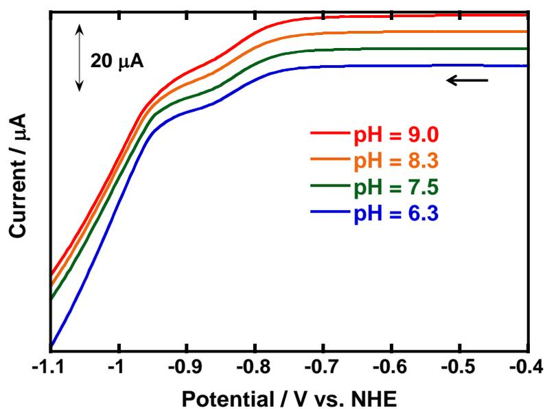
**Fig. S2** SWVs of  $1 \cdot 2\text{H}_2\text{O}$  (0.5 mM) in an aqueous 0.1 M  $\text{KNO}_3$  solution under Ar atmosphere, using a glassy carbon working electrode, a platinum wire counter electrode, and a saturated calomel reference electrode, where the pH of each solution was adjusted simply by adding KOH without using any buffer reagents.
