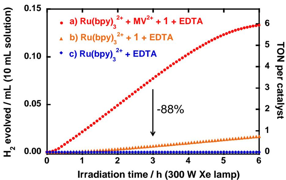
**Fig. S4** Photochemical H<sub>2</sub> production from an aqueous acetate buffer solution (0.03 M CH<sub>3</sub>COOH and 0.07 M CH<sub>3</sub>COONa; pH 5.0; 10 mL) containing EDTA (30 mM; disodium salt) and [Ru(bpy)<sub>3</sub>](NO<sub>3</sub>)<sub>2</sub>·3H<sub>2</sub>O (0.04 mM), a) with MV(NO<sub>3</sub>)<sub>2</sub> (2.0 mM) and 1·2H<sub>2</sub>O (0.1 mM), b) with 1·2H<sub>2</sub>O (0.1 mM), or c) without acceptor and catalyst, under Ar atmosphere at 20 °C.
