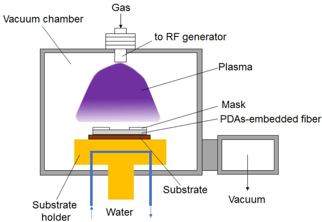
Figure S3. Schematic representation of plasma induced polymerization.
