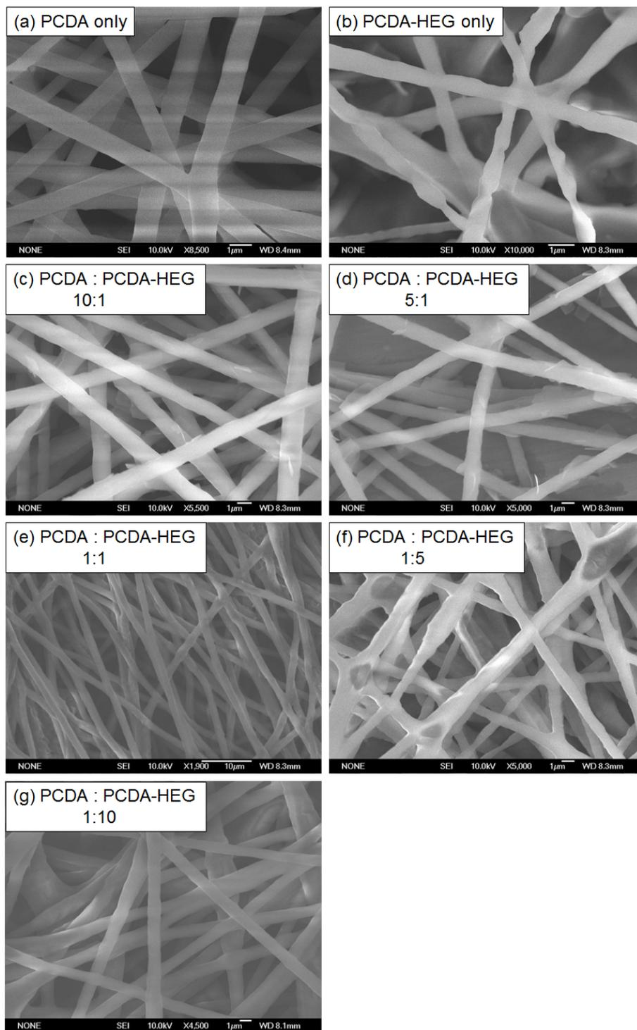
Figure S4. SEM images of PCDA, PCDA-HEG and their combinations embedded fibers.
