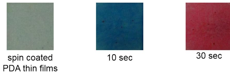
Figure S5. Time-dependent color changes of spin coated PDA thin films in the presence of plasma (Radio frequency powers: 200W, Argon gas pressure: 21 mTorr)
