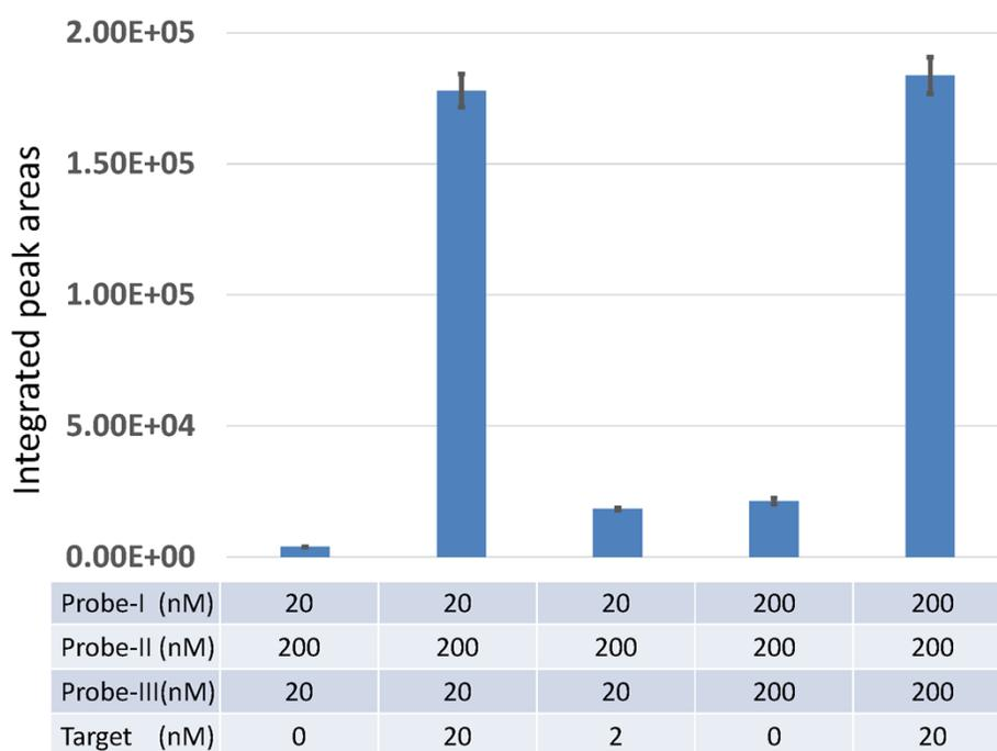
Figure S1. Comparison of the dAMP signals obtained with different compositions of the ternary DNA probe solution.
