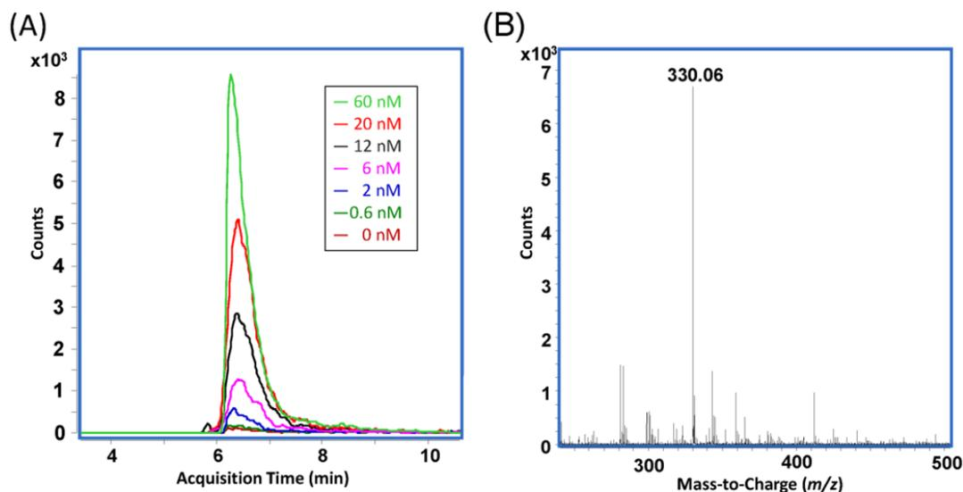
Figure S4. (A) The elected ion chromatograph (EIC) of  $m/z$  330.06 (dAMP) at different concentration of thrombin. (B) The MS spectrum of the EIC peak in the detection of 20 nM thrombin.
