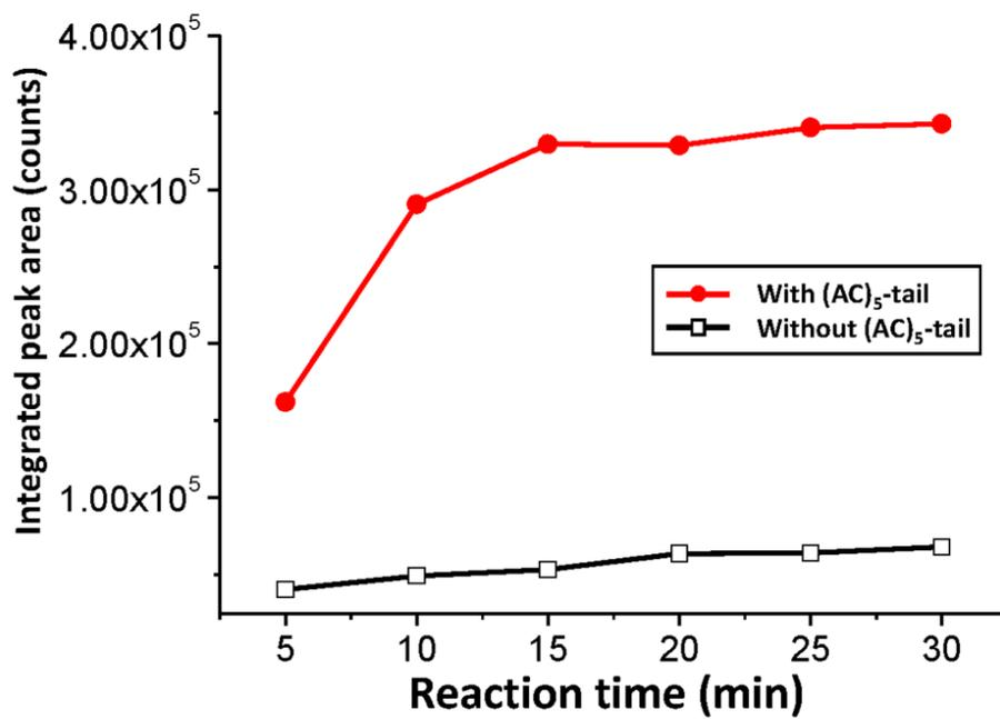
Figure S2. Time curves of dAMP signals obtained by using Probe-II with/without the (AC)<sub>5</sub>-tail for the amplification reaction.
