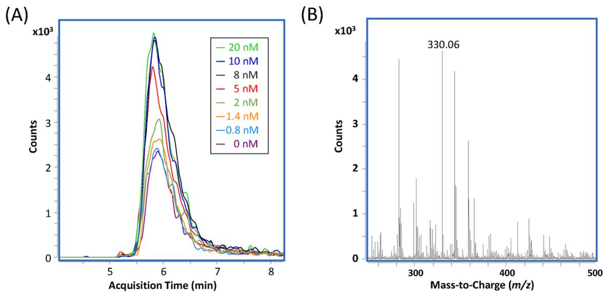
Figure S3. (A) The elected ion chromatograms (EIC) of  $m/z$  330.06 (dAMP) at different concentration of target ssDNA. (B) The MS spectrum of the EIC peak in the detection of 60 nM target ssDNA.
