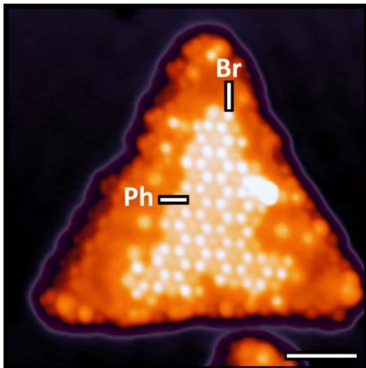
STM images showing the ordered network of Br atoms and phenyl groups that forms at high coverage on the Co nanoparticle surfaces. The phenyl molecules appear as dimmer protrusions in the matrix of brighter round features, which are the Br atoms. Scale bar = 3 nm.
