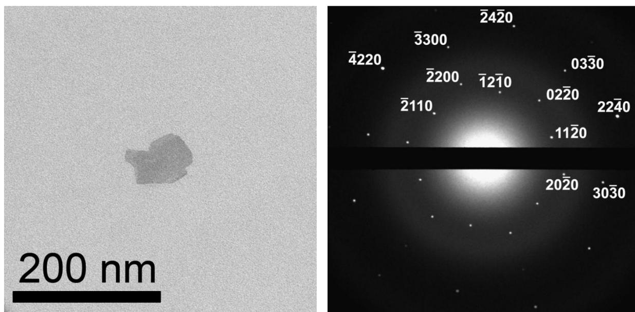
**Figure S4.** Single colloidal particle and corresponding electron diffraction pattern (electron beam is normal to the particle basal plane) with marked strontium hexaferrite reflections.
