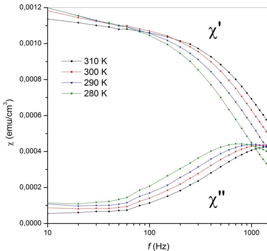
**Figure S6.** AC-susceptibility measurements of F680 sample (field amplitude of 4 Oe).
