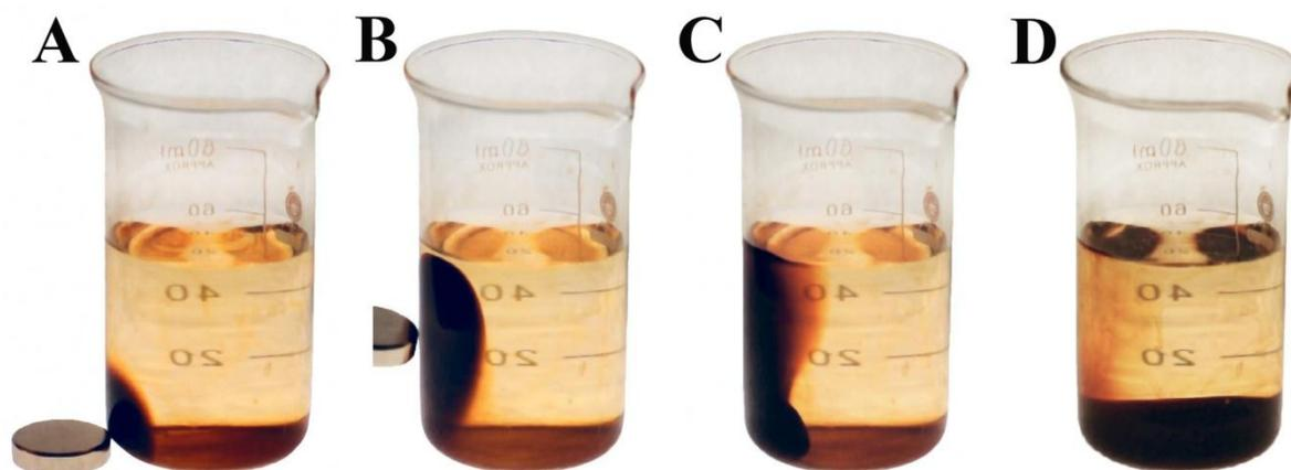
**Figure S2.** Separation of concentrated liquid phase in FA750 sample after prolonged exposure to inhomogeneous magnetic field of NdFeB magnet (A). Behavior of the phase in the presence (B) and absence (C, D) of the magnetic field.
