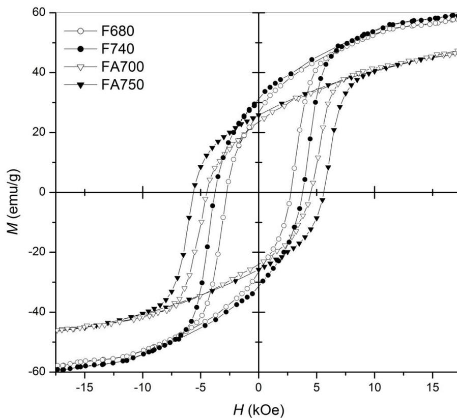
**Figure S5.** Hysteresis loops of dried colloidal particles.
