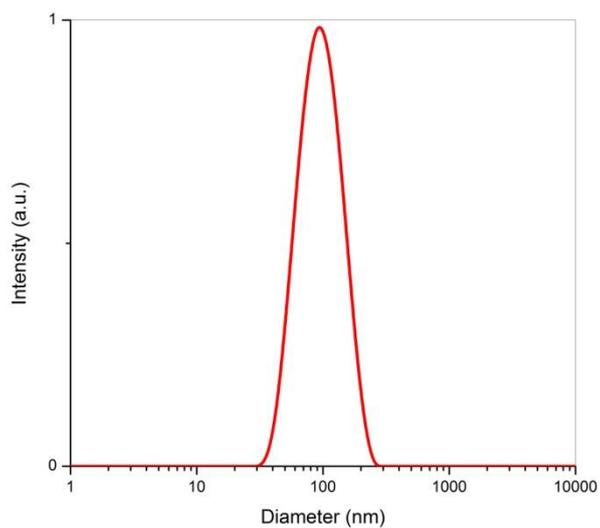
**Figure S5a.** Intensity distribution of hydrodynamic diameters of colloidal particles in FA750 sample (DLS).
