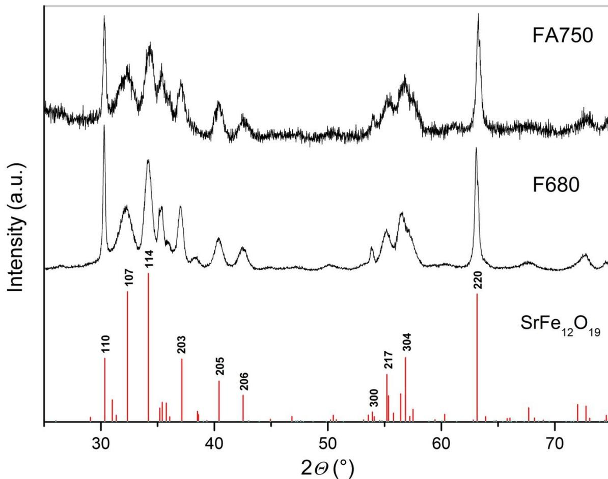
**Figure S3.** XRD patterns of dried colloidal particles in comparison with  $\text{SrFe}_{12}\text{O}_{19}$  diffraction lines (PDF- 84-1531).
