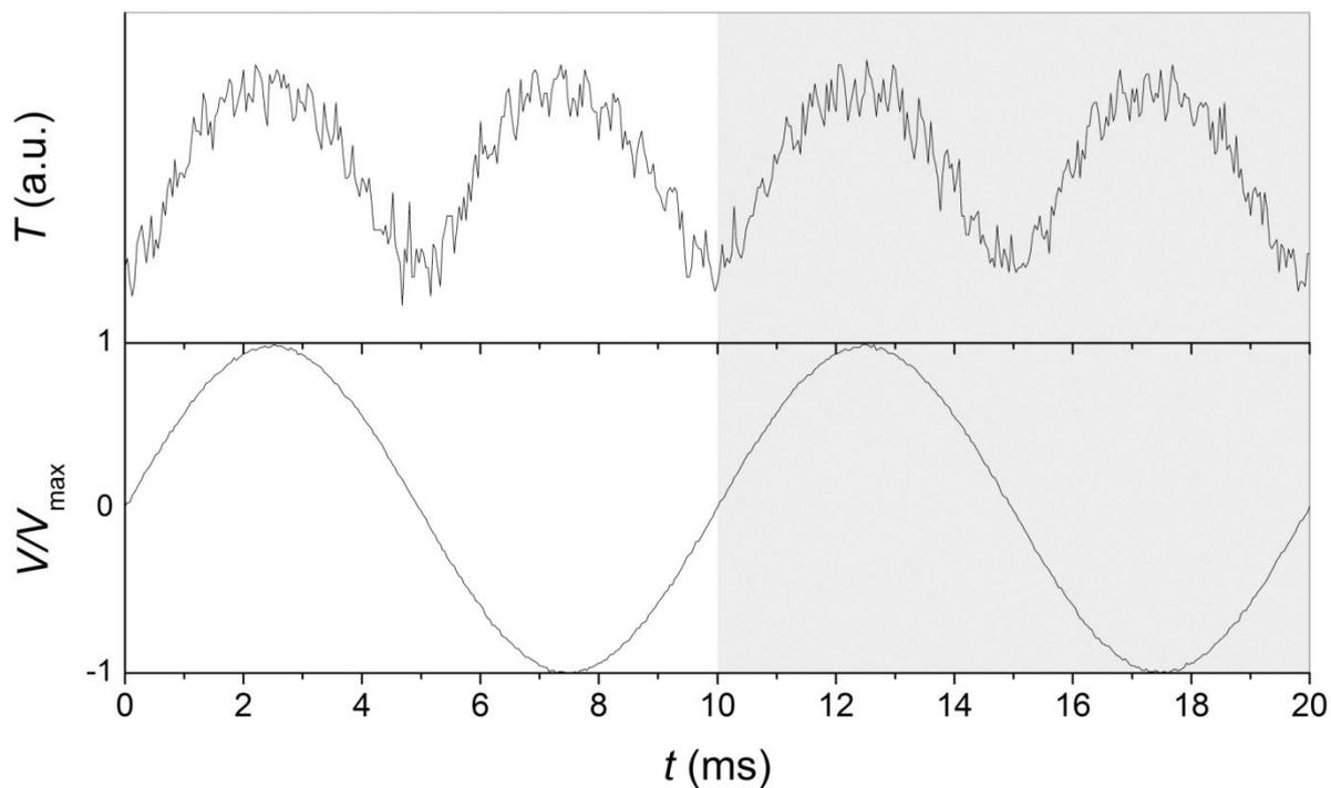
**Figure S7.** Optical oscillations under an alternating magnetic field (100 Hz, 4 Oe). Optical response changes with doubled frequency compared with the supplied voltage of Helmholtz coil.
