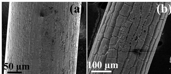
**Figure S5.** The FE-SEM images of (a) Ti thread, (b) a Ti thread coated with TiO<sub>2</sub> nanotube arrays.
