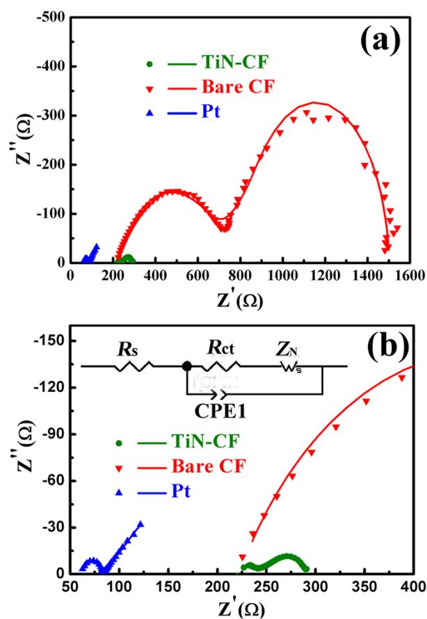
**Figure S7.** (a) Nyquist plots of the symmetric cells with two identical counter electrodes of TiN-CF, Pt wire or bare CF in the measured frequency range from 100 kHz to 100 mHz. The spectra for both cells were measured in the same redox active electrolyte; (b) the enlargement of (a). The symbols are experimental data, and the solid lines are fitted results according to the inset equivalent circuit.
