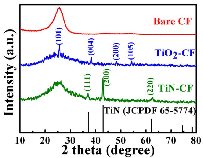
**Figure S3.** XRD patterns collected from TiN-CF, TiO<sub>2</sub>-CF and bare CF.
