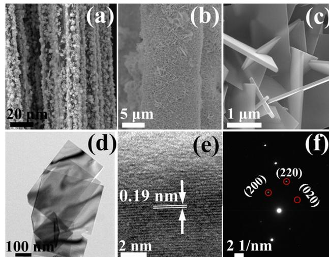
**Figure S1.** (a), (b) and (c) low magnification and high magnification FE-SEM images of  $\text{TiO}_2$  nanoplates, (d) TEM image, (e) HRTEM image, and (f) SAED recorded from  $\text{TiO}_2$  nanoplate.
