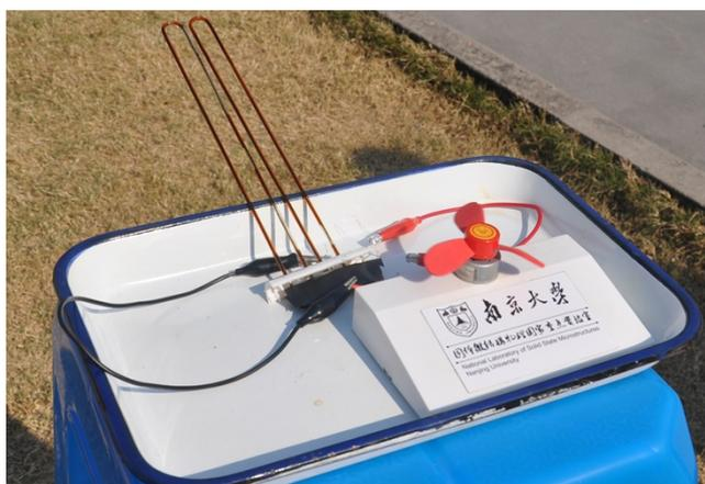
**Figure S10.** A screenshot of Movie S1 which shows a solar cell module enables to easily drive a small fan motor in an outdoor sunlight.
