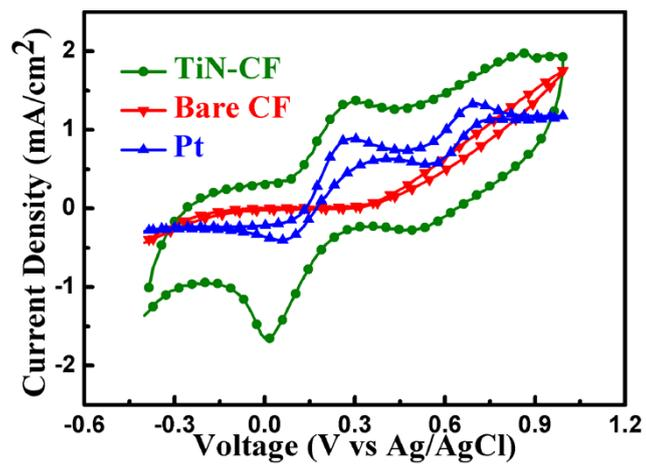
**Figure S6.** Cyclic voltammograms for TiN-CF, Pt wire electrodes and bare CF.
