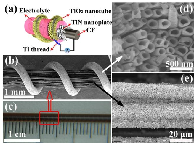
**Figure S9.** (a) schematic setup of the FDSSC, (b) FE-SEM image of FDSSC, (c) photograph of the FDSSC, (d) FE-SEM image of TiO<sub>2</sub> nanotube growing on Ti thread, and (e) FE-SEM image of TiN nanoplates coating on CF.
