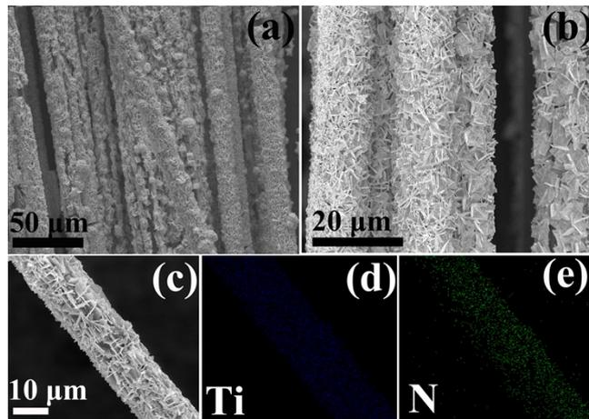
**Figure S2.** (a), (b), and (c) low magnification and high magnification FE-SEM images of TiN nanoplates; (d) and (e) TiN-CF was characterized using EDX elemental mapping.
