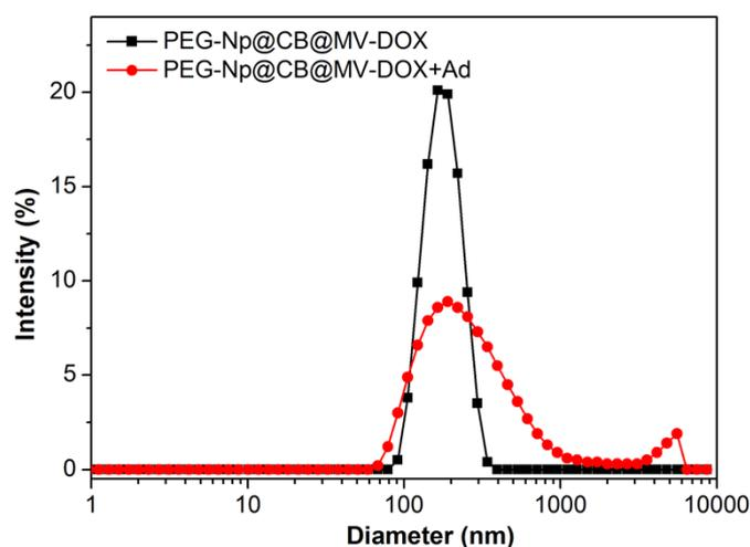
Figure S10. DLS plots of supramolecular micelles before and after treated with adamantane(Ad) for 5 min.
