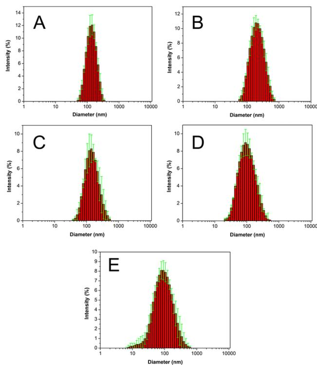
Figure S15. DLS plots of supramolecular prodrug micelles in water (A), 1M PBS (B), 20X dilution (C), DMEM (D) and DMEM with 10 % FBS (E).
