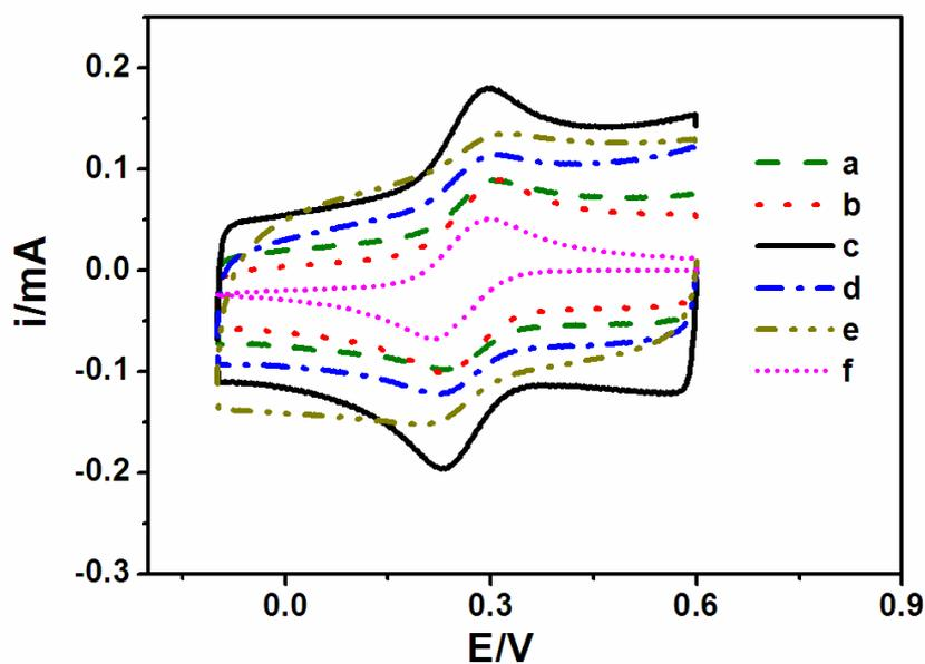
**Fig. S8** CVs of different electrodes in 0.50 mM  $Fe(CN)_6^{3-}$  containing 1.0 M KCl: (a) PCCM<sub>900</sub>-3%/GCE, (b) PCCM<sub>900</sub>-2%/GCE, (c) PCCM<sub>900</sub>-1%/GCE, (d) PCCM<sub>900</sub>-0.5%/GCE, (e) PCCM<sub>900</sub>-0%/GCE, and (f) unmodified GCE.
