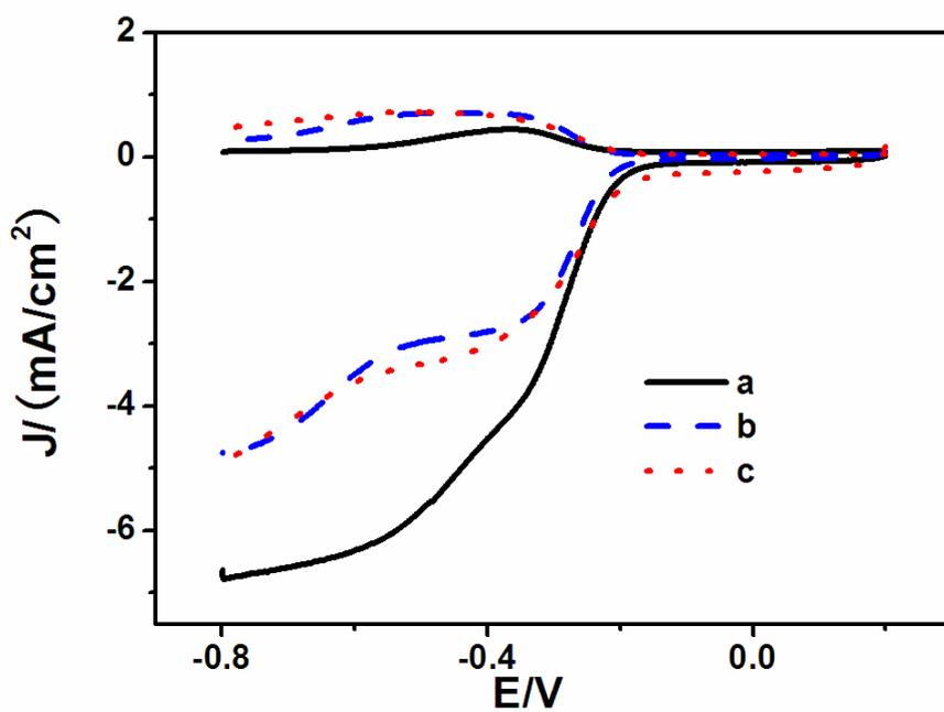
**Fig. S10** RRDE voltammograms of (a) PCCM<sub>900</sub>-1%/GCE, (b) g-PCCM<sub>900</sub>-1%/GCE, and (c) PCCM<sub>900</sub>-0%/GCE in O<sub>2</sub>-saturated 0.10 M KOH at a scan rate of 5 mV/s, a rotation rate of 1600 rpm, and the Pt ring electrode is polarized at 0.2 V (vs Ag/AgCl).
