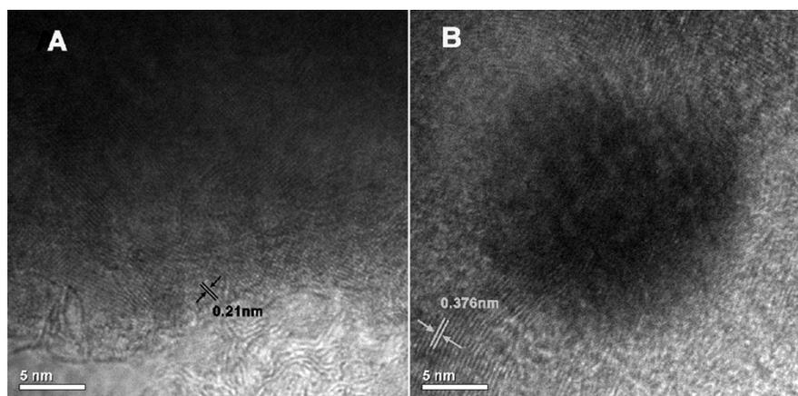
**Fig. S2** High resolution TEM images of the PCCM<sub>900</sub>-1%. The distances of 0.21 and 0.376 nm are corresponding to (211) and (011) crystal planes of Fe<sub>3</sub>C phase, respectively.
