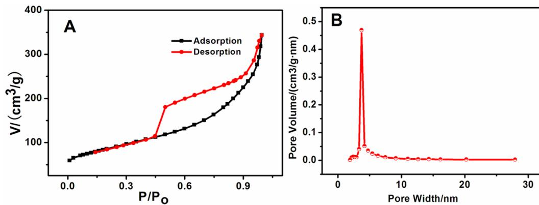
**Fig. S4** (A) N<sub>2</sub> adsorption-desorption isotherm of the PCCM<sub>900</sub>-1% composite and (B) the pore size distribution of the composite from BJH plot.
