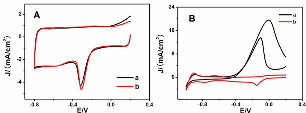
**Fig. S9** CVs of (A) PCCM<sub>900</sub>-1%/GCE and (B) Pt/C/GCE in O<sub>2</sub>-saturated 0.10 M KOH solution (a) with and (b) without 1.0 M CH<sub>3</sub>OH. Scan rate is 50 mV/s.
