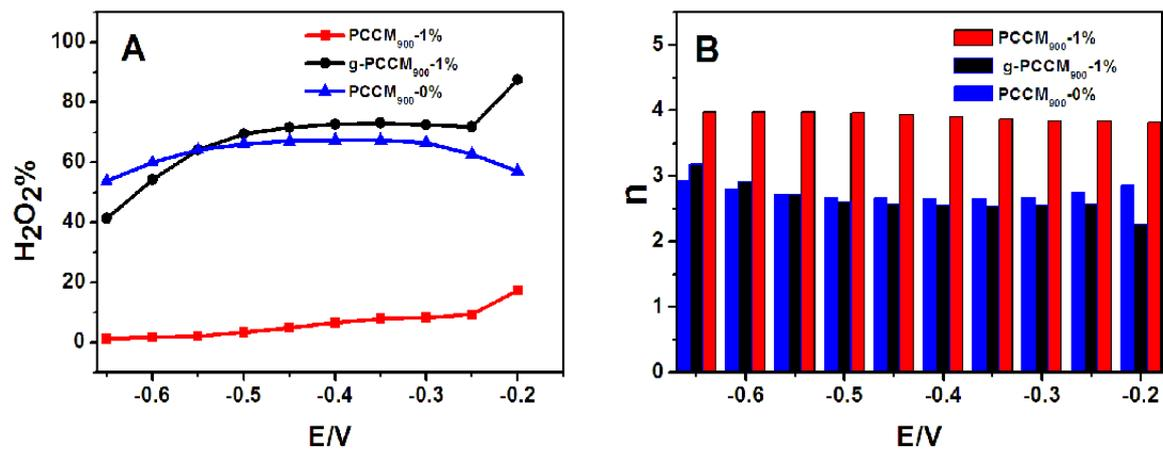
**Fig. S11** (A) H<sub>2</sub>O<sub>2</sub> yield of the PCCM<sub>900</sub>-1%/GCE, g-PCCM<sub>900</sub>-1%/GCE, and PCCM<sub>900</sub>-0%/GCE. (B) Electron transfer number (n) of the PCCM<sub>900</sub>-1%/GCE, g-PCCM<sub>900</sub>-1%/GCE, and PCCM<sub>900</sub>-0%/GCE.
