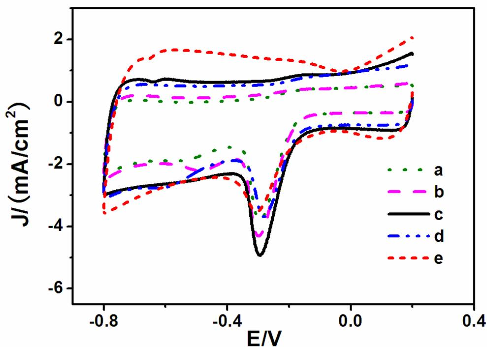
**Fig. S7** CVs on different modified GCE in  $O_2$ -saturated 0.10 M KOH: (a) PCCM<sub>900</sub>-3%/GCE, (b) PCCM<sub>900</sub>-2%/GCE, (c) PCCM<sub>900</sub>-1%/GCE, (d) PCCM<sub>900</sub>-0.5%/GCE, and (e) PCCM<sub>900</sub>-0%/GCE. Scan rate is 50 mV/s.
