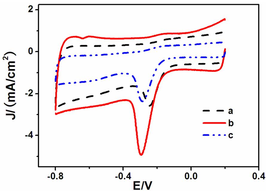
**Fig. S6** Cyclic voltammograms (CVs) tested in O<sub>2</sub>-saturated 0.10 M KOH: (a) PCCM<sub>800</sub>-1%/GCE, (b) PCCM<sub>900</sub>-1%/GCE, and (c) PCCM<sub>1000</sub>-1%/GCE. Scan rate is 50 mV/s. (vs Ag/AgCl)
