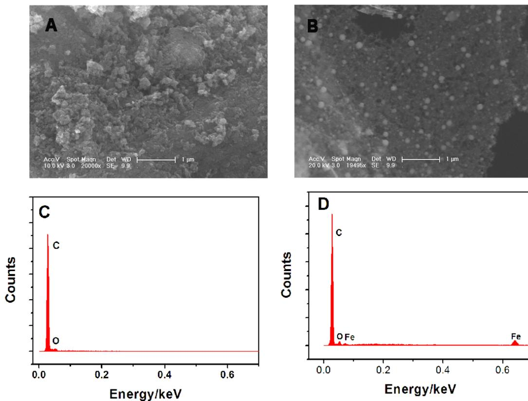
**Fig. S5** SEM images of (A) g-PCCM<sub>900</sub>-1%, (B) PCCM<sub>900</sub>-1% and corresponding EDAX spectra of (C) g-PCCM<sub>900</sub>-1% and (D) PCCM<sub>900</sub>-1%.
