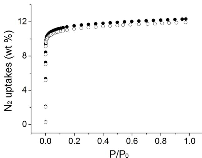
**Figure S9.** N<sub>2</sub> adsorption and desorption isotherms of NENU-3-Ina before (solid disc) and after (hollow circle) be rinsed with hot water and ethanol.
