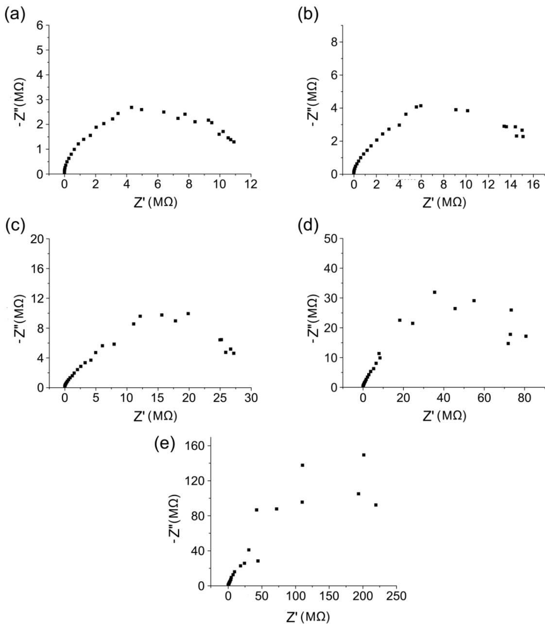
**Figure S2.** Nyquist plots of HKUST-1 at 70% RH and various temperatures (a) 90 °C, (b) 80 °C, (c) 70 °C, (d) 60 °C, (e) 50 °C.
