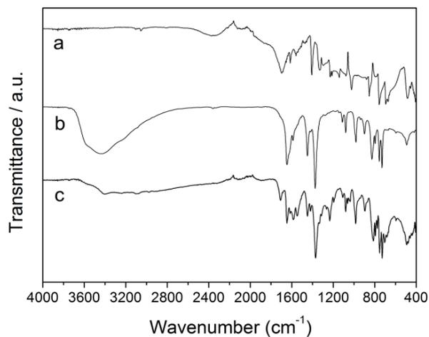
**Figure S7.** FTIR spectrum of (a) Isonicotinic acid, (b) NENU-3, and (c) NENU-3-Ina.
