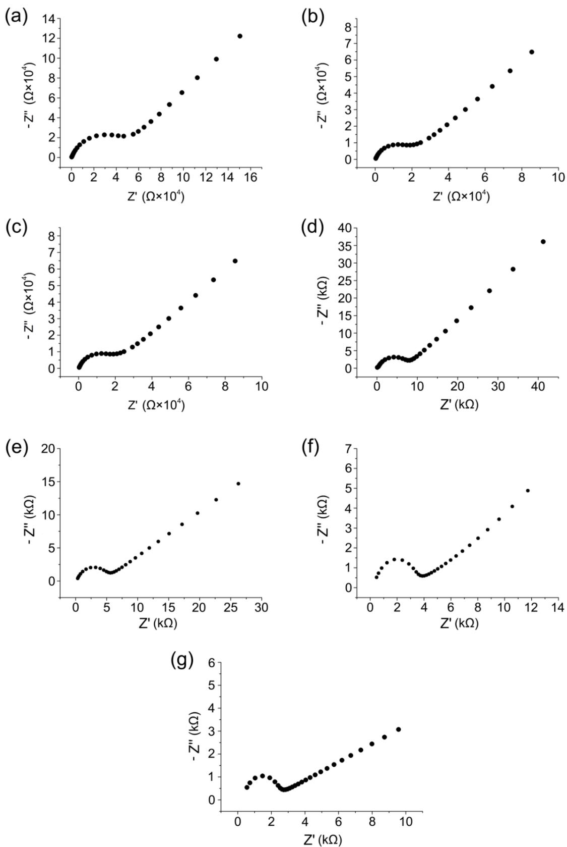
**Figure S1.** Nyquist plots of NENU-3 at 70% RH and various temperatures (a) 25 °C, (b) 40 °C, (c) 50 °C, (d) 60 °C, (e) 70 °C, (f) 80 °C, (g) 90 °C.
