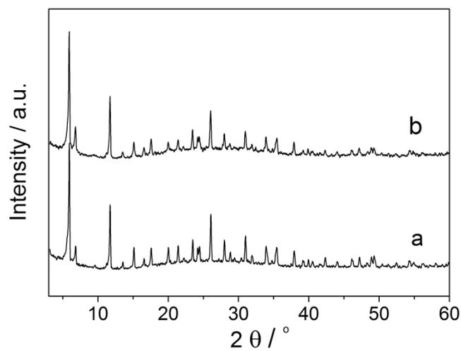
**Figure S5.** PXRD patterns of NENU-3 before (a) and after (b) the impedance measurement.
