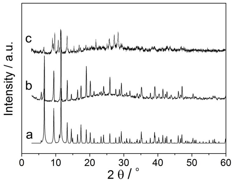
**Figure S3.** PXRD patterns of HKUST-1 (a) simulated, (b) as-synthesized, and (c) the sample after be exposed in water vapor for ~2 hours.
