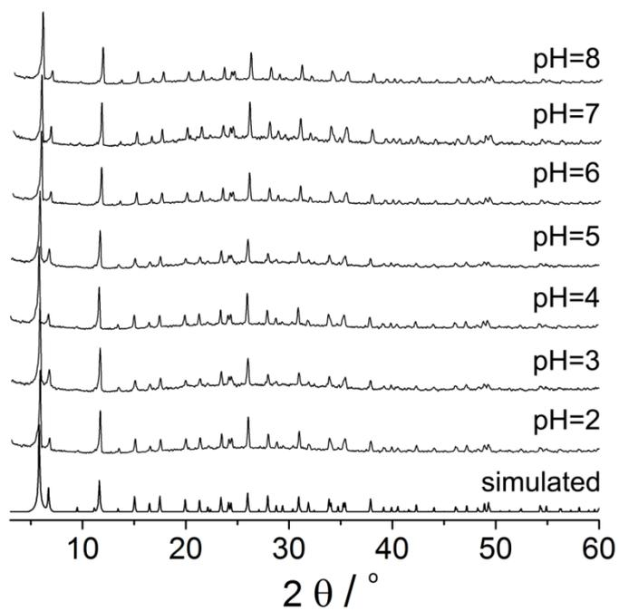
**Figure S4.** PXRD patterns of NENU-3 after having been soaked in aqueous solution with different pH value for 1 week, the pH value is adjusted by HCl or NaOH.
