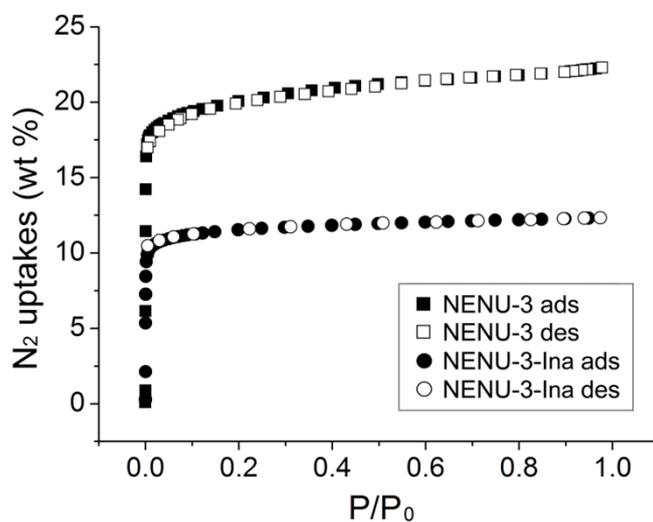
**Figure S8.** N<sub>2</sub> adsorption and desorption isotherms of NENU-3 and NENU-3-Ina
