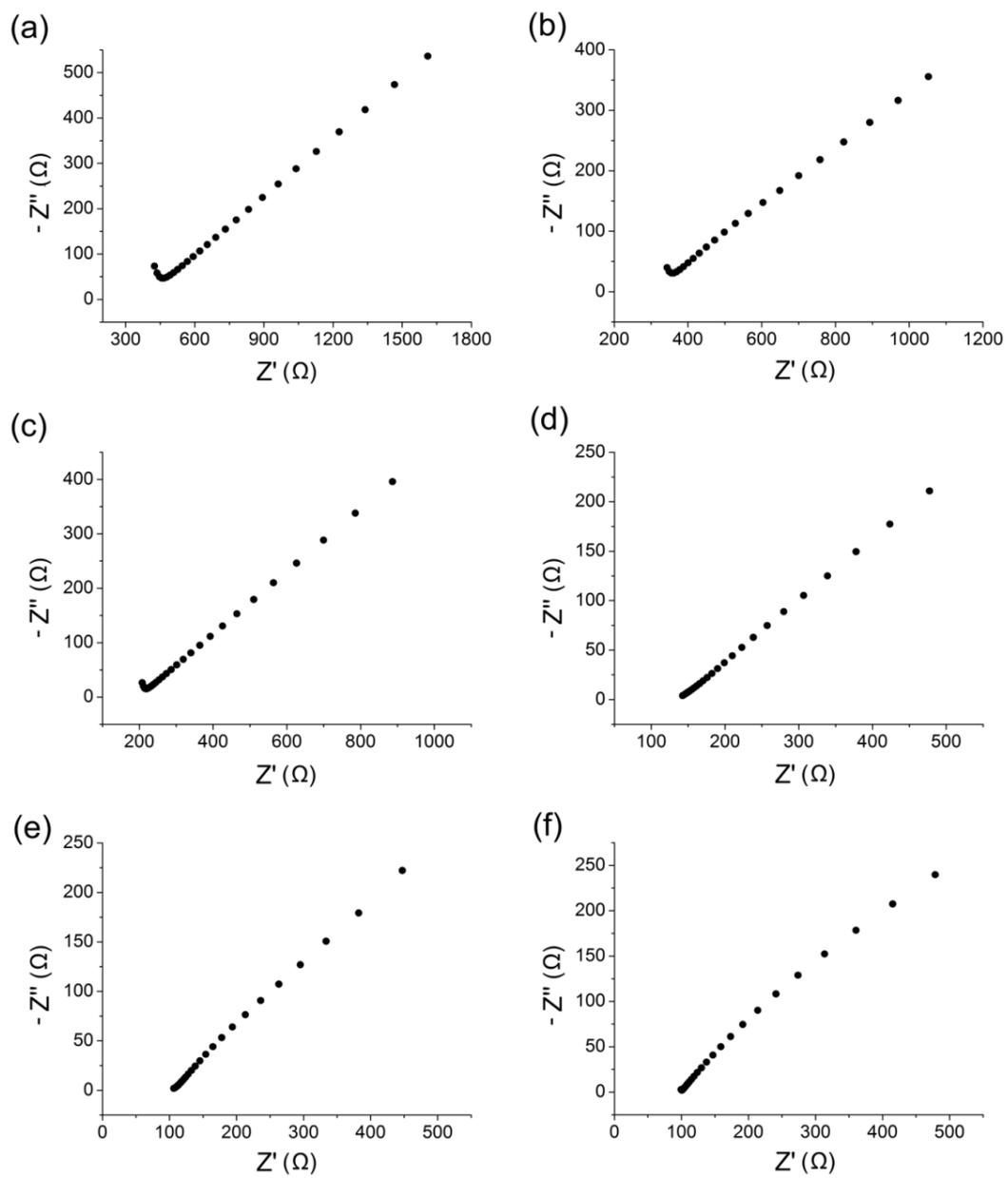
**Figure S10.** Nyquist plots of NENU-3-Ina at at 70% RH and various temperatures (a) 40 °C, (b) 50 °C, (c) 60 °C, (d) 70 °C, (e) 80 °C, (f) 90 °C.
