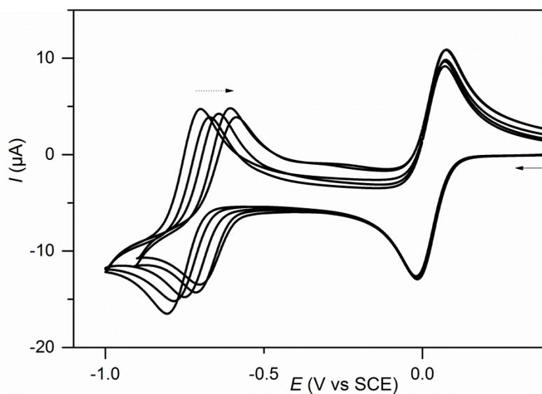
**Figure S2.** Cyclic voltammograms of TCQ (0.5 mM) on a glassy carbon electrode in a solution of TBAPF<sub>6</sub> (0.1 M) in acetonitrile in the absence and in the presence of increasing iodo-perfluorobenzene (**3**) concentrations (from left to right: 0; 0.5, 5, 25; 50 mM). Scan rate 0.1 V/s.
