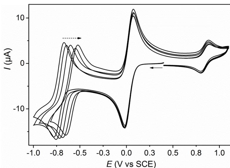
**Figure S1.** Cyclic voltammograms of TCQ (0.5 mM) and Os(bpy)<sub>3</sub>PF<sub>6</sub> (0.12 mM) on a glassy carbon electrode in a solution of TBAPF<sub>6</sub> (0.1 M) in acetonitrile in the absence and in the presence of increasing concentrations of iodo-perfluorohexane (1) (from left to right: 0, 0.5, 5, 25, 50 mM). Scan rate 0.1 V/s.
