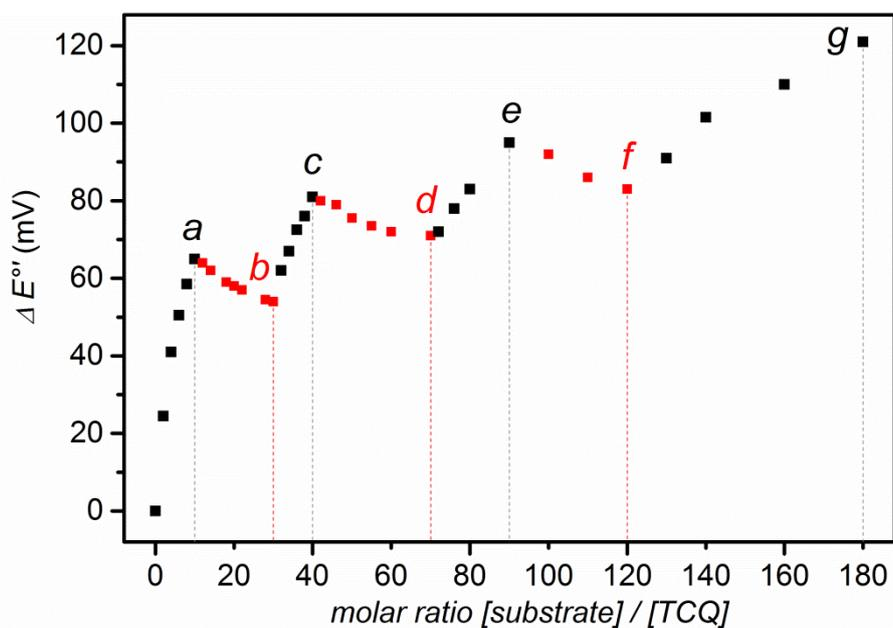
**Figure S4.** Potential shift of the second voltammetric wave of TCQ (0.5 mM) in a solution of 0.1 M TBAPF<sub>6</sub> in acetonitrile before and after adding successively the XB-donor **1** (black squares; a: 10 eq., c: 10 eq., e: 20 eq., g: 60 eq.) and the Lewis base Cl<sup>-</sup> in the form of TBACl (red squares; b: 20 eq., d: 30 eq., f: 30 eq.).
