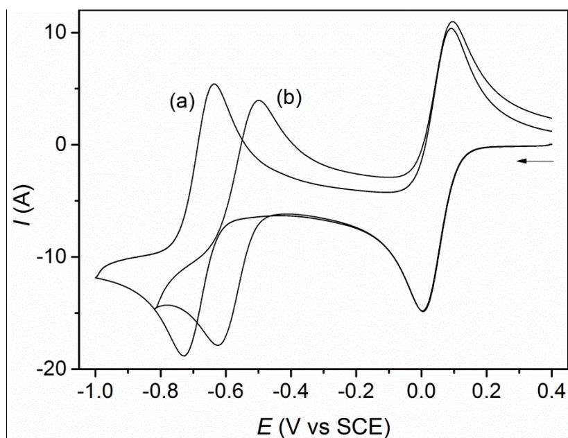
**Figure S6.** Cyclic voltammograms of TCQ (0.5 mM) on a glassy carbon electrode in a solution of tetramethylammonium hexafluorophosphate at 0.1 M in acetonitrile in the absence (a) and in the presence (b) of 100 equiv. of iodo-perfluorohexane (**1**) concentrations. Scan rate 0.1 V/s.
