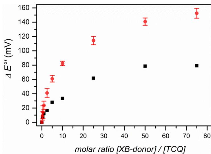
**Figure S3.** Dependence of the potential shift  $\Delta E^{\circ'}$  corresponding to the second reduction step of TCQ at 0.5 mM (red dots, including standard deviations) and 0.1 mM (black squares) on the concentration of the XB-donor **1** at 298 K.
