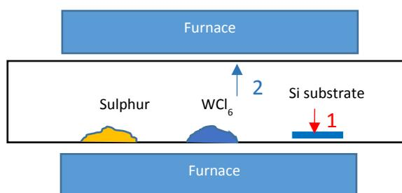
Figure S1. Schematic diagram of CVD setup
