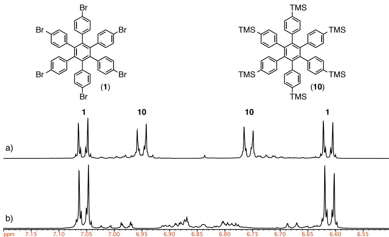
**Figure S2.** Partial <sup>1</sup>H NMR spectra (500 MHz, CDCl<sub>3</sub>, 298 K) of the crude mixture obtained by quenching with TMSCl 2.5 min after removal of the cooling bath a) in the absence of MesBr, b) in the presence of MesBr.
