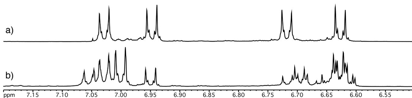
**Figure S1.** Partial <sup>1</sup>H NMR spectra (500 MHz, CDCl<sub>3</sub>, 298 K) of the crude mixture obtained in the lithiation of compound **1** with a) *t*-BuLi (6 equiv.) or b) PhLi (3 equiv.).
