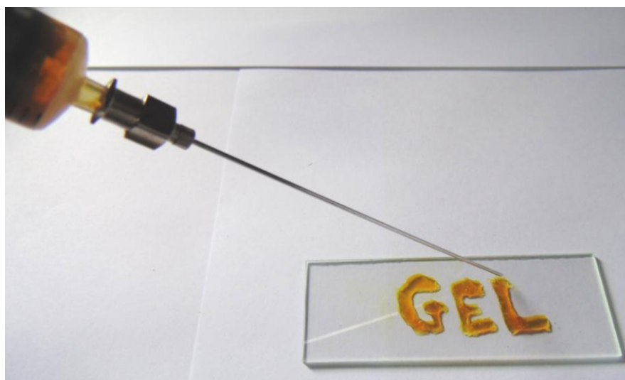
Figure S9. Injectability of the hydrogel has been demonstrated by writing different alphabetical letters on top of a glass plate.
