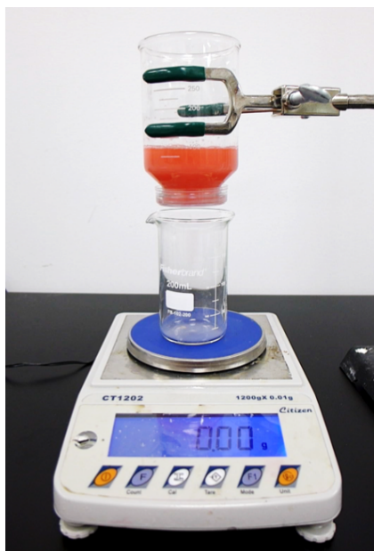
Figure S3: Experimental setup of water/oil emulsion separation.
