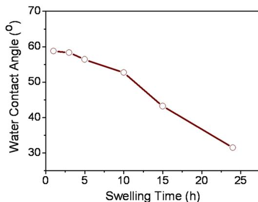
**Figure S7.** Water contact angles of PS-*b*-P2VP films subjected to ethanol swelling at 50 °C for different durations.
