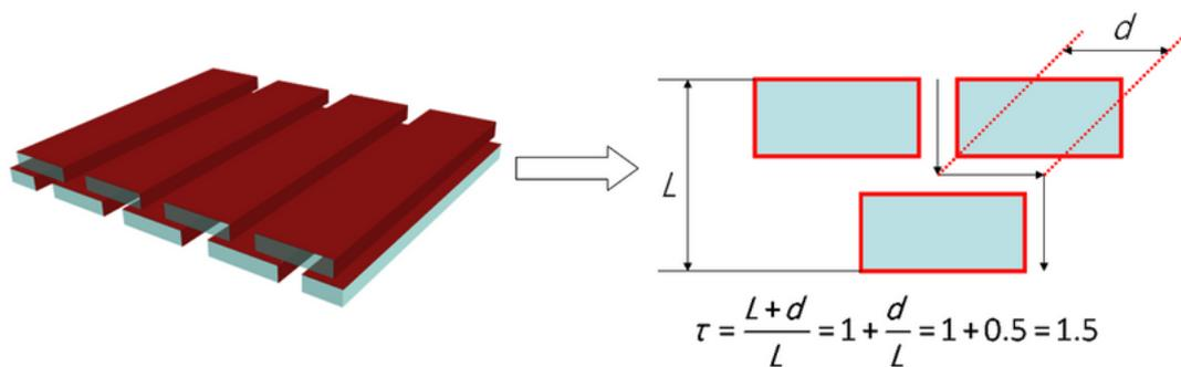
**Figure S12.** The value of  $d$  is nearly one half of the thickness of the selective layer from the analysis by SEM.
