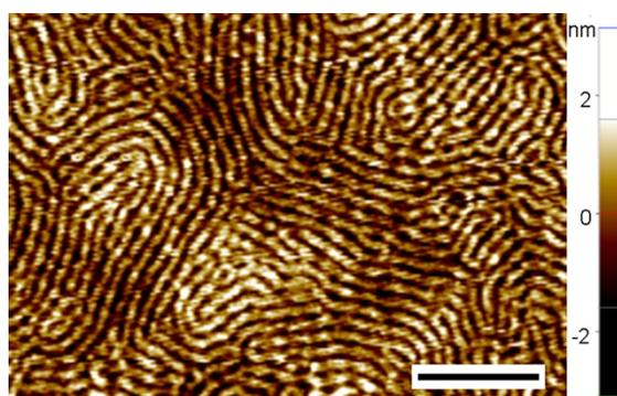
**Figure S1.** The AFM height image of the TCE-annealed BCP film with the P2VP cylinders parallel to the substrate surface. The scale bar is 400 nm.
