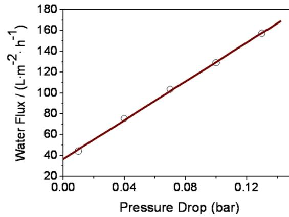
**Figure S11.** The fit-linear curve of flux and transmembrane pressure of the composite membrane with the BCP selective layer subjected to ethanol swelling at 50 °C for 3 h.
