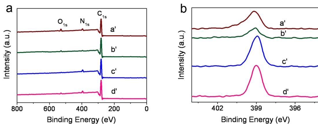
**Figure S8.** (a) XPS wide-spectra; (b) The corresponding enlarged spectra. XPS detailed the peak of  $N_{1s}$  of PS-*b*-P2VP films subjected to different treatments: the as-coated film subjected to ethanol swelling at 50 °C for 3 h (a'), and the TCE-annealed film before (b') and after ethanol swelling at 50 °C for 3 h (c') and 24 h (d').
