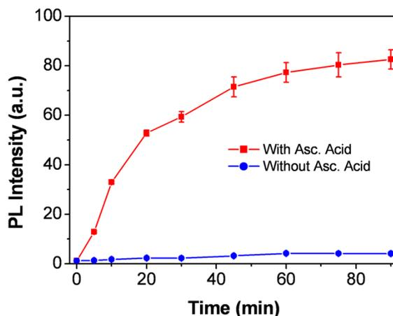
**Figure S8.** PL intensity at 480 nm of cRGD-TPE-Pt-DOX (10  $\mu\text{M}$ ) in the presence (red) and absence (blue) of ascorbic acid (Asc. Acid, 1 mM) from 0 to 90 min. Data represent mean values  $\pm$  standard deviation,  $n = 3$ .
