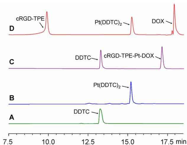
**Figure S6.** HPLC spectra showing the reaction of diethyldithiocarbamate (DDTC) with cisplatin and reduced Pt(IV) prodrug: (A) DDTC alone; (B) the product for reaction between DDTC and cisplatin; (C) the mixture of DDTC and cRGD-TPE-Pt-DOX; (D) the products for the reaction between DDTC and cRGD-TPE-Pt-DOX ( $10 \mu\text{M}$ ) after treatment with 1 mM ascorbic acid for 12 h.
