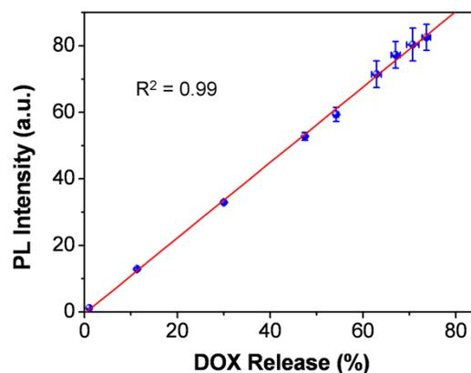
**Figure S12.** Correlation between released DOX to emitted fluorescence of cRGD-TPE ( $\lambda_{\text{ex}} = 320$  nm,  $\lambda_{\text{em}} = 480$  nm) upon reduction of cRGD-TPE-Pt-DOX with ascorbic acid.
