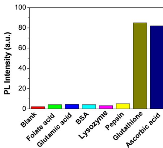
**Figure S9.** Fluorescence response of cRGD-TPE-Pt-DOX (10  $\mu\text{M}$ ) toward 1.0 mM folate acid, glutamic acid, bovine serum albumin (BSA), lysozyme, pepsin, glutathione or ascorbic acid in DMSO/PBS ( $v/v = 1/199$ ).
