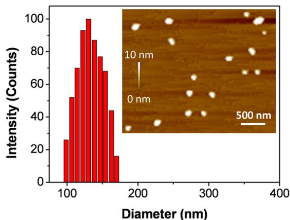
**Figure S2.** Laser light scattering data and AFM image (inset) of cRGD-TPE (10  $\mu$ M) in DMSO/PBS (v/v = 1/199).
