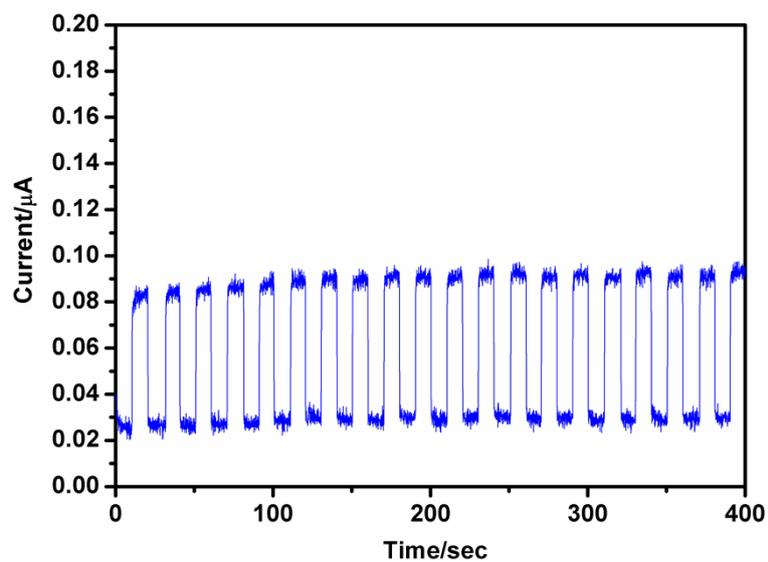
Fig. S2 Photocurrent stability of the proposed  $\text{Hg}^{2+}$  transducer to 300 pM  $\text{Hg}^{2+}$
