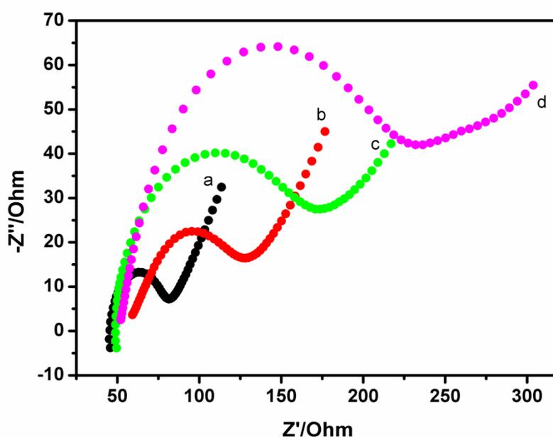
**Figure S1** EIS of (a) bare Au electrodes (b) after MSO probe immobilization and MCH blocking, (c) after CdS QDs anchoring (d) after combining the  $\text{Hg}^{2+}$  corresponding to 500 pM. The EIS measurements are carried out in 0.1 M KCl containing 5.0 mM  $\text{K}_3\text{Fe}(\text{CN})_6/\text{K}_4\text{Fe}(\text{CN})_6$  (1:1). The frequency range was between 1 and 100 000 Hz with an applied voltage of 5 mV.
