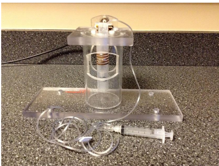
Figure 1. The radio-frequency solenoid coil, the reactor, and the injection line.
