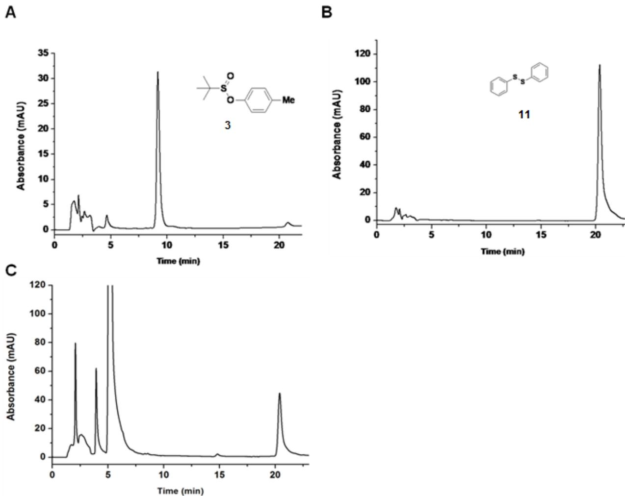
**Figure S1.** (a) Authentic p-tolyl 2-methylpropane-2-sulfinate (**3**, 100 μM); (b) Authentic sample of thiophenol disulfide (**11**); (c) **3** (100 μM) was treated with thiophenol (10 equiv) and incubated at 37 °C. The reaction mixture after 30 min of was analyzed by HPLC and shows complete disappearance of **3** with formation of **11**.
