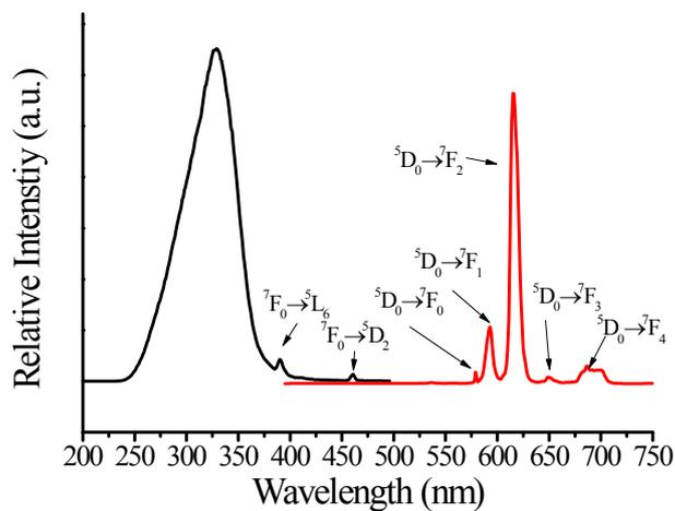
**Figure S5.** The excitation (black) and emission spectra (red) of MOF-253-Eu (the  $\lambda_{em} = 614$  nm and the  $\lambda_{ex} = 330$  nm).
