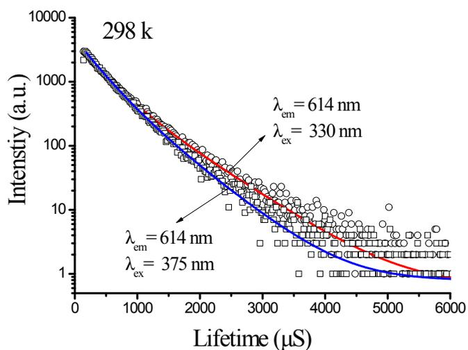
**Figure S6.** The decay curve of MOF-253-Eu-TTA, the red is obtained under  $\lambda_{em} = 614$  nm and the  $\lambda_{ex} = 330$  nm, the blue is obtained under  $\lambda_{em} = 614$  nm and the  $\lambda_{ex} = 375$  nm, which is record under 298 k.
