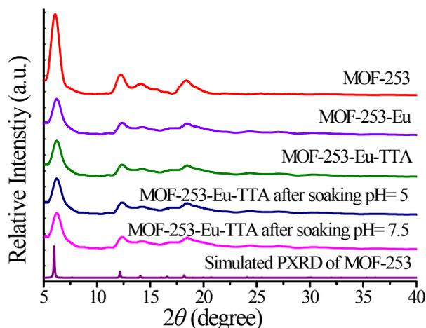
**Figure S1.** PXRD for MOF-253, MOF-253-Eu, MOF-253-Eu-TTA, MOF-253-Eu-TTA after soaking pH = 5 and MOF-253-Eu-TTA after soaking pH = 7.7, the PXRD of MOF-253 is consistent with reported literature.<sup>S1</sup>
