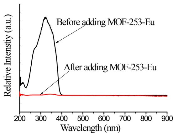
**Figure S10.** The UV-Vis spectra of the solution before adding MOF-253-Eu and after adding MOF-253-Eu
