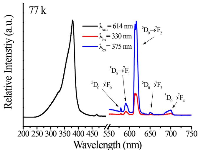
**Figure S7.** The excitation spectrum ( $\lambda_{em} = 614$  nm) of MOF-253-Eu-TTA (black) and the emission spectra of MOF-253-Eu-TTA,  $\lambda_{ex} = 330$  nm (red) and  $\lambda_{ex} = 375$  nm (blue), which is record under 77 k.
