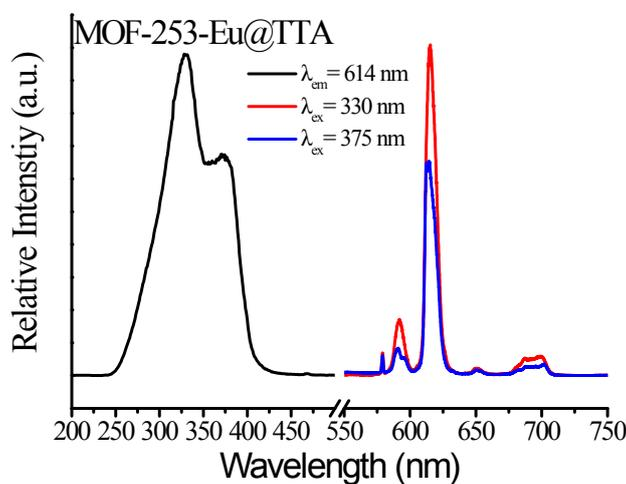
**Figure S11.** The excitation spectrum ( $\lambda_{em} = 614$  nm) of MOF-253-Eu-TTA (black) and the emission spectra of MOF-253-Eu-TTA,  $\lambda_{ex} = 330$  nm (red) and  $\lambda_{ex} = 375$  nm (blue)
