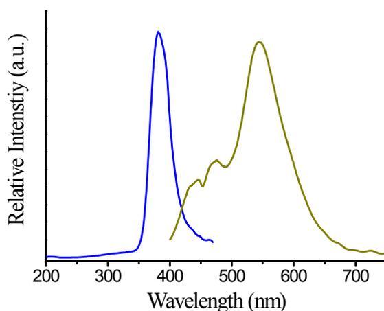
**Figure S8.** The excitation (blue) and PL spectra (yellow) of MOF-253 ( $\lambda_{em} = 550$  nm and  $\lambda_{ex} = 385$  nm).
