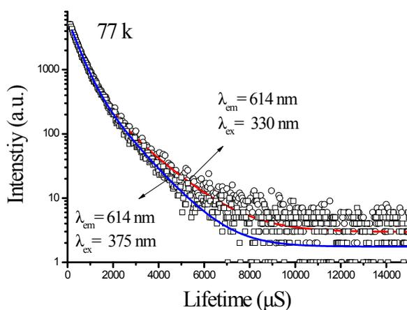
**Figure S9.** The decay curve of MOF-253-Eu-TTA, the red is obtained under  $\lambda_{em} = 614$  nm and the  $\lambda_{ex} = 330$  nm, the blue is obtained under  $\lambda_{em} = 614$  nm and the  $\lambda_{ex} = 375$  nm, which is record under 77 k.
