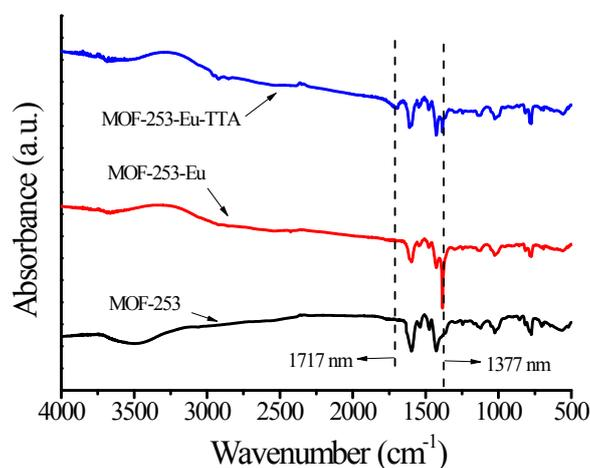
**Figure S3.** FT-IR spectra of MOF-253, MOF-253-Eu and MOF-253-Eu-TTA.
