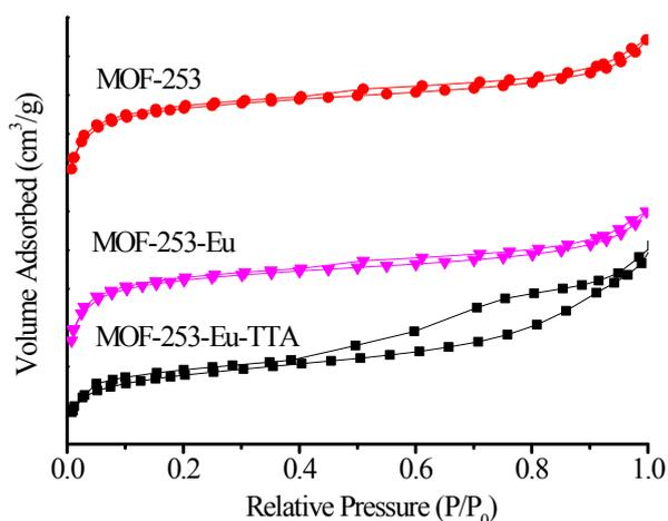
**Figure S2.** N<sub>2</sub> adsorption-desorption isotherms of MOF-253, MOF-253-Eu and MOF-253-Eu-TTA, the Langmuir surface areas of MOF-253, MOF-253-Eu and MOF-253-Eu-TTA were calculated to be 1188, 728 and 287 m<sup>2</sup>/g, the Langmuir surface areas of MOF-253 is consistent with reported literature<sup>S3</sup>
