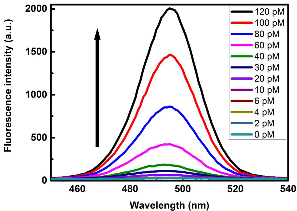
**Figure S 6** The fluorescence spectra of the assay system as a function of the amount of target DNA.
