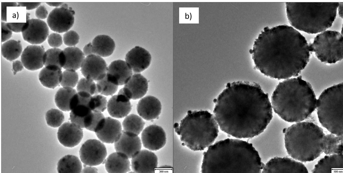
**Figure S 2** TEM images of MNP-Ag presented with 300-nm (a) and 100-nm (b) scale bar.
