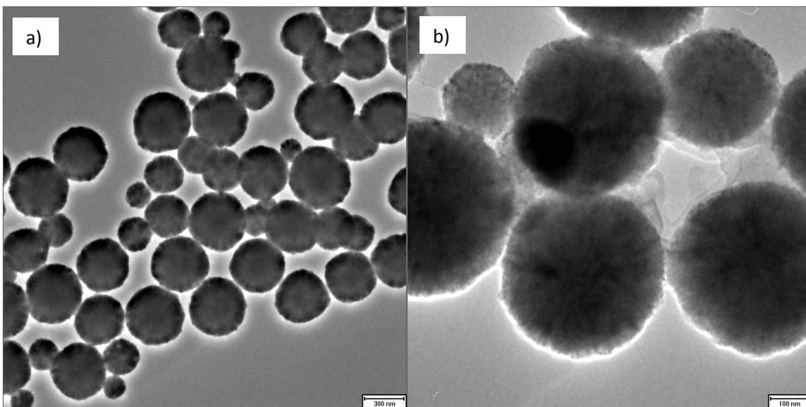
**Figure S 1** TEM images of MNPs presented with 300-nm (a) and 100-nm (b) scale bar. The diameter of MNP is  $(186 \pm 8)$  nm ( $n = 50$ ).
