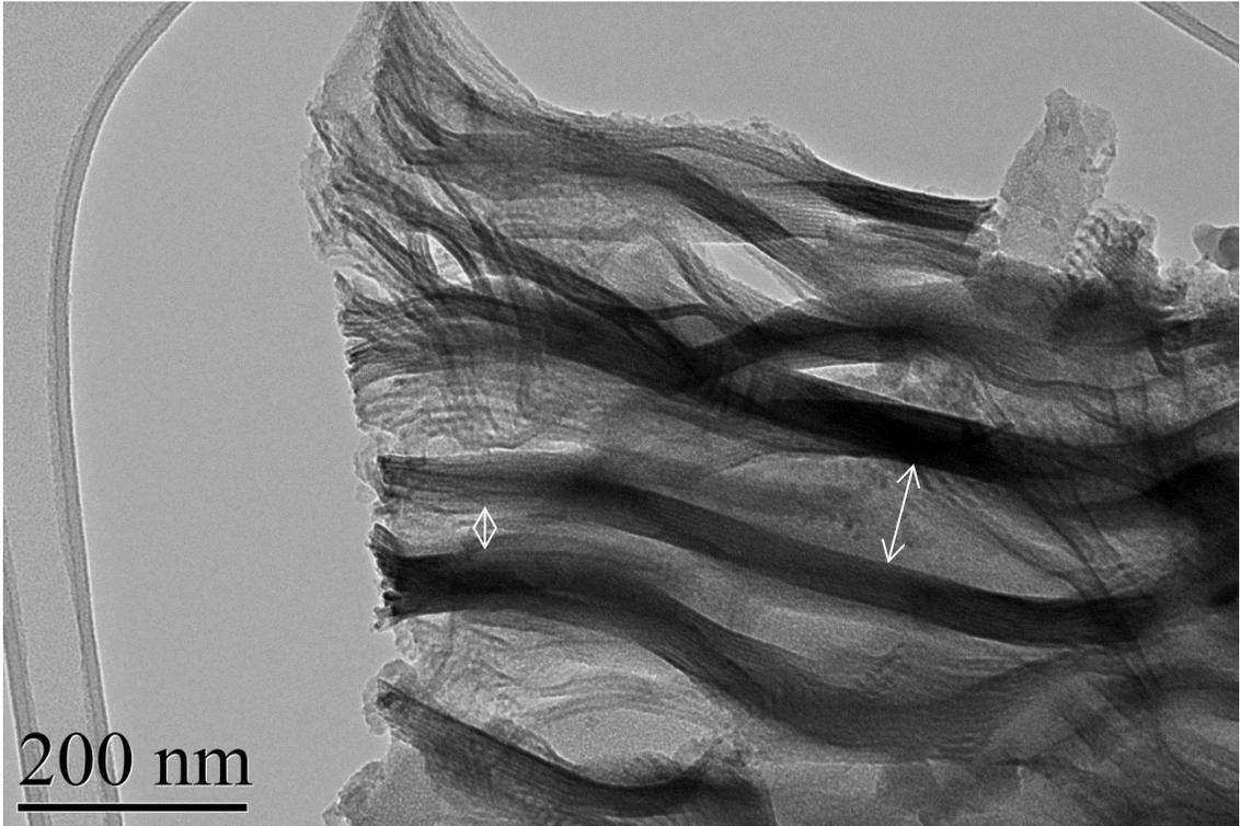
S5: TEM image of the mesostructuration state of macropore walls core
