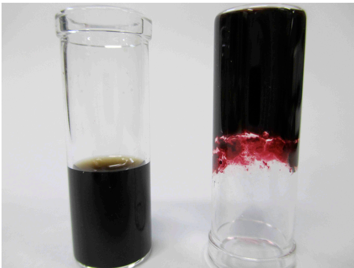
Fig. S2 Photographic image of GO dispersion (left vial) and TAI-GO gel (right vial) prepared by adding 2.1 mg PDI to 2 ml of hot GO aqueous dispersion ( 2.0 \text{ mg ml}^{-1} , \sim 70^\circ\text{C} ). \sim 15 \text{ min.} of sonification resulted in gelation.
