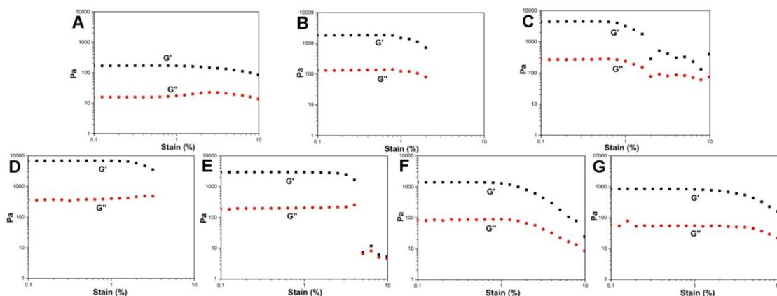
**Fig. S-12.** Rheological measurement with the mode of dynamic strain sweep at the frequency of 1 rad/s and strain of 0.1% for the gel of Nap-FFYGK-CA with different equivalent of melamine: A (0.25 equiv), B (0.5 equiv), C(1 equiv), D(2 equiv), E(4 equiv), F(8 equiv), G(16 equiv).
