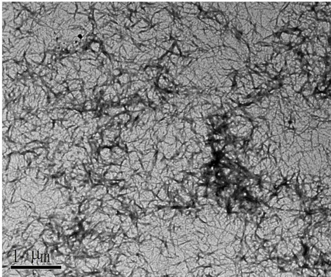
**Fig. S-8.** A representative TEM image of a gel of Nap-FFYGK-CA with 8 equivalent of melamine
