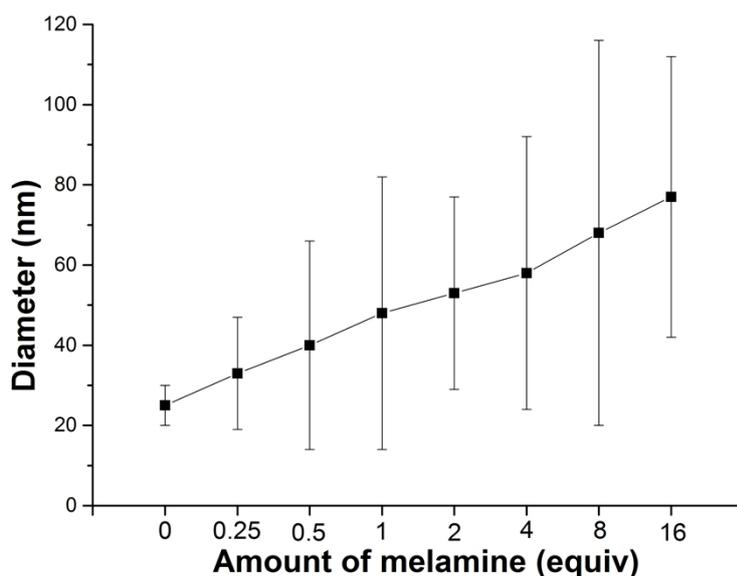
**Fig. S-9.** Diameter of the fibers in the gels of Nap-FFYGK-CA with different amount of melamine (more than 50 nanofibers in several TEM images were used and their diameter was calculated to obtain the mean diameter)
