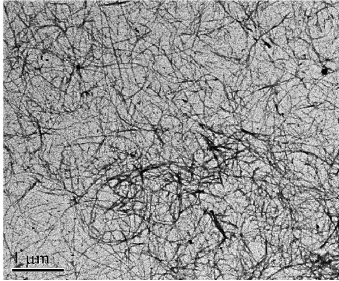
**Fig. S-7.** A representative TEM image of a gel of Nap-FFYGK-CA with 1 equivalent of melamine
