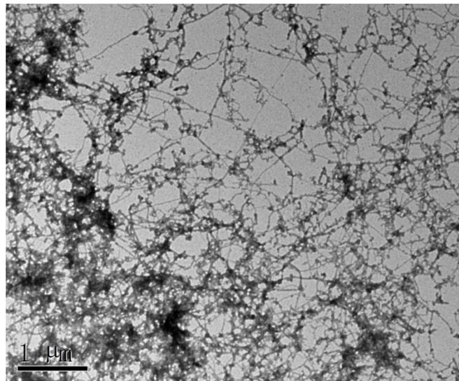
**Fig. S-6.** A representative TEM image of a gel of Nap-FFYGK-CA with 0.5 equivalent of melamine
