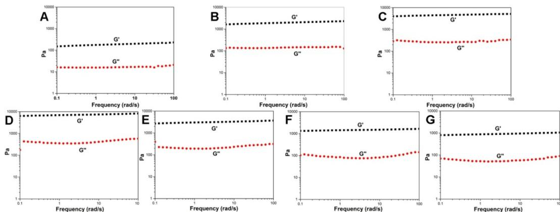
**Fig. S-11.** Rheological measurement with the mode of dynamic frequency sweep at the frequency of 1 rad/s and strain of 0.1% for the gel of Nap-FFYGK-CA with different equivalent of melamine: A (0.25 equiv), B (0.5 equiv), C(1 equiv), D(2 equiv), E(4 equiv), F(8 equiv), G(16 equiv)
