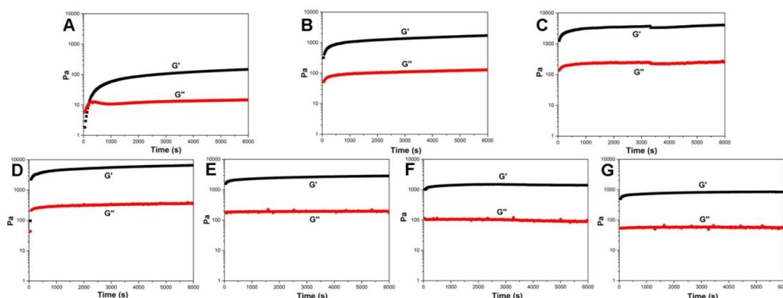
**Fig. S-10.** Rheological measurement with the mode of dynamic time sweep at the frequency of 1 rad/s and strain of 0.1% for the gels of Nap-FFYGK-CA with different equivalent of melamine: A (0.25 equiv), B (0.5 equiv), C (1 equiv), D (2 equiv), E (4 equiv), F (8 equiv), G (16 equiv)
